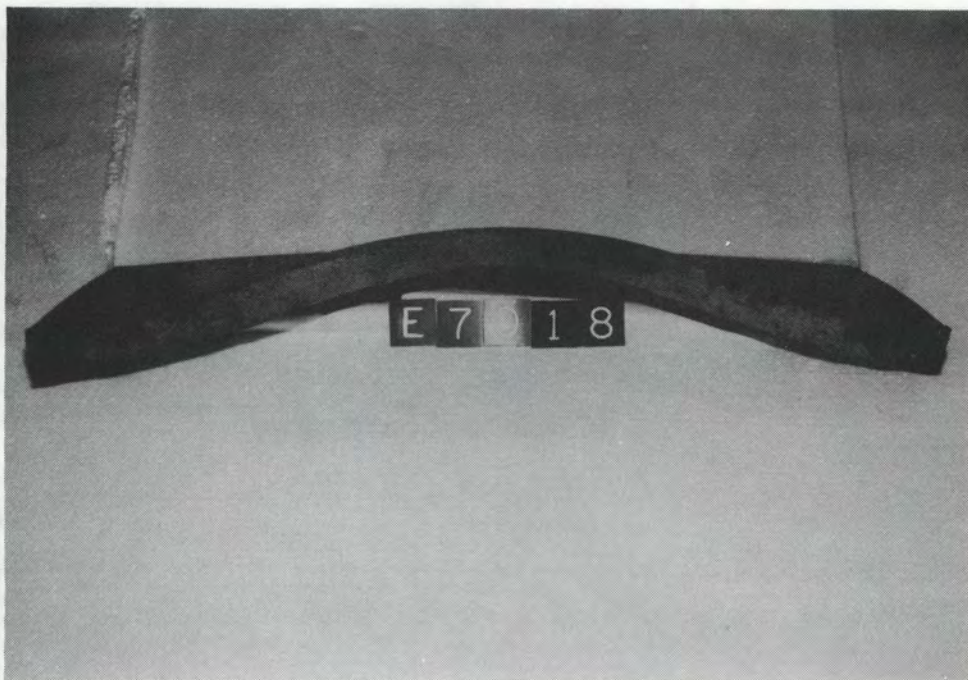
Figure 3: View of completely fractured E7018 test panel
