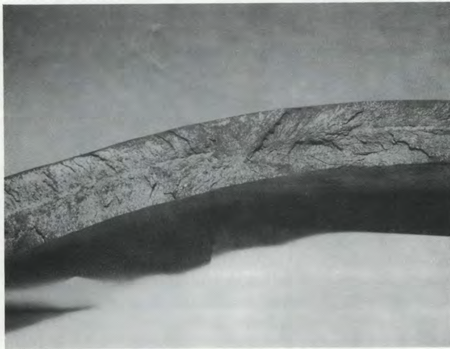
Figure 14: Fracture surface of E7018 weld showing chevron fracture pattern
