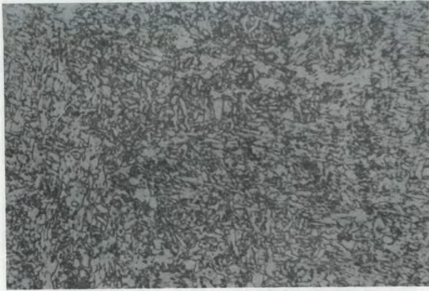
Figure 9: Microstructure of E9018M weld metal showing fine acicular ferrite (500X)
