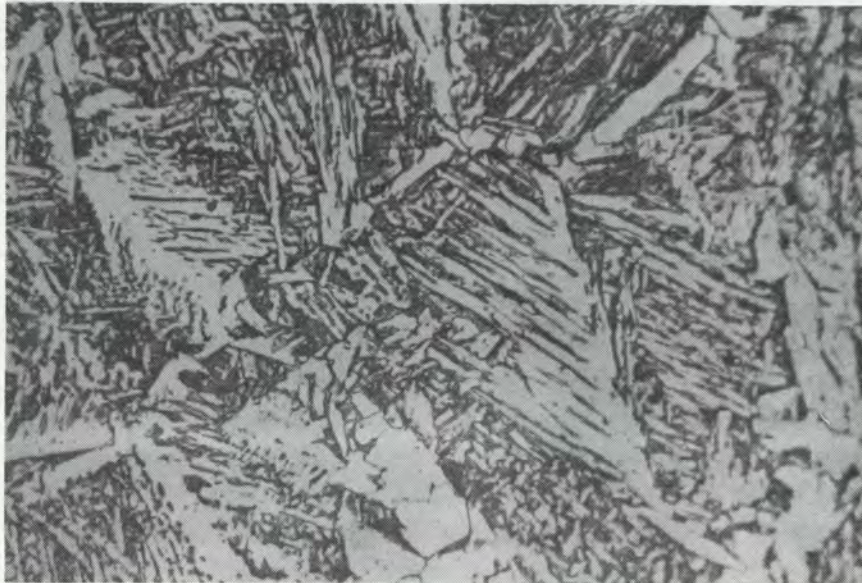
Figure 12: Microstructure of 70S1 Narrow Gap weld metal showing coarse acicular ferrite and side plate ferrite (500X)
