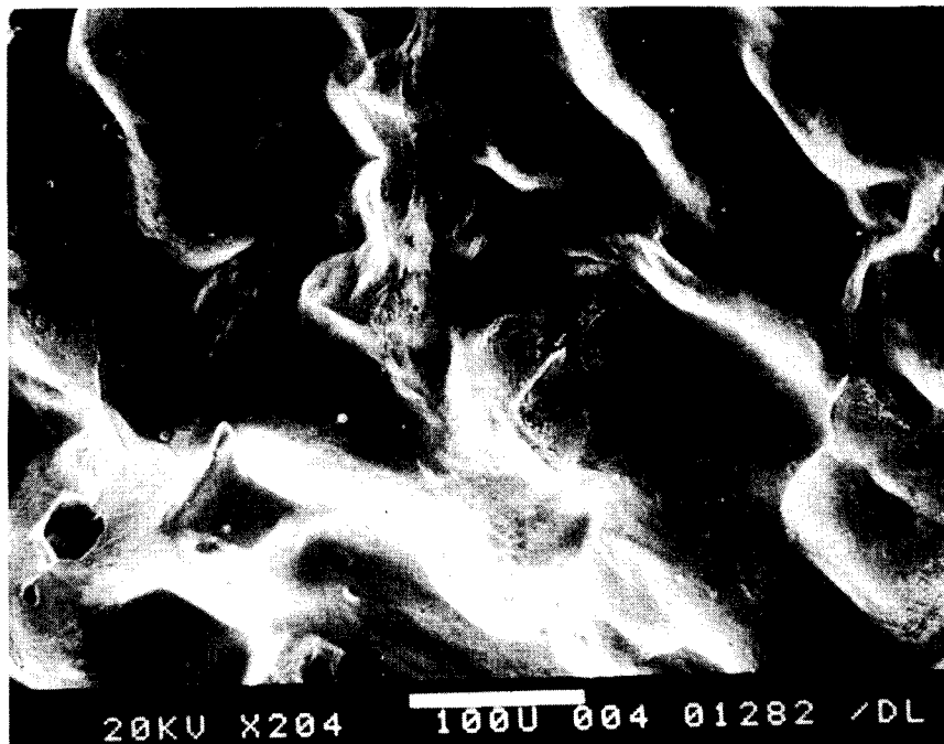
Figure 32: Eroded surface of niobium modified 70/30 copper nickel alloy parent metal. (X204)
