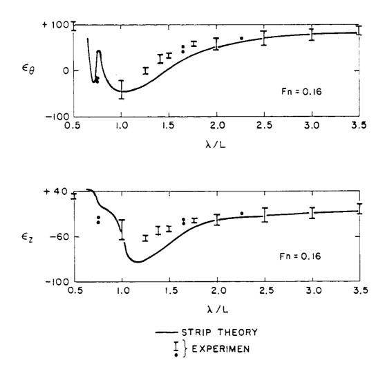
Figure 1 - Measured and Predicted Pitch and Heave Phase Angles for the Fishing Vessel of Reference 19
