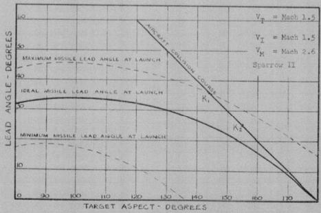
Fig. 4. Lead Angle vs Target Aspect.
