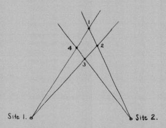
Fig. 20. - Ambiguity Introduced by Triangulation of bearings on Two Targets.
