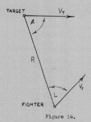
Figure 14 shows the interceptor and target separated by distance R . The rate of closure of the aircraft
