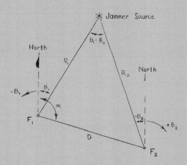
Fig. 18. - Range by Triangulation - Two Aircraft.
