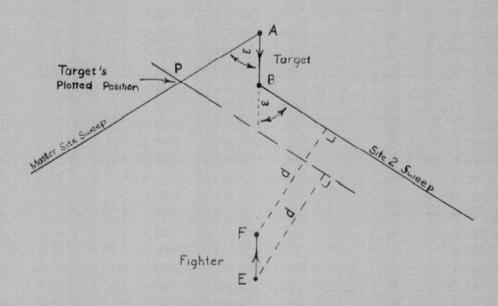
Fig. 22. - Plotting error from asynchronous radars.
