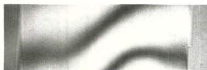
Figure 42. Beam Shearing Interferogram after a liquid gate with proper index matching liquid.
