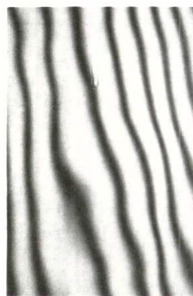
Figure 38. Beam Shearing Interferogram after reflection on two poor mirrors
