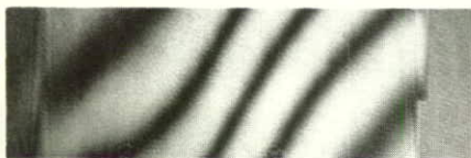
Figure 41. Beam Shearing interferogram after an empty liquid gate.
