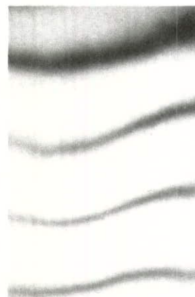
Figure 35. Beam Interferogram after reflection on one good quality mirror.
