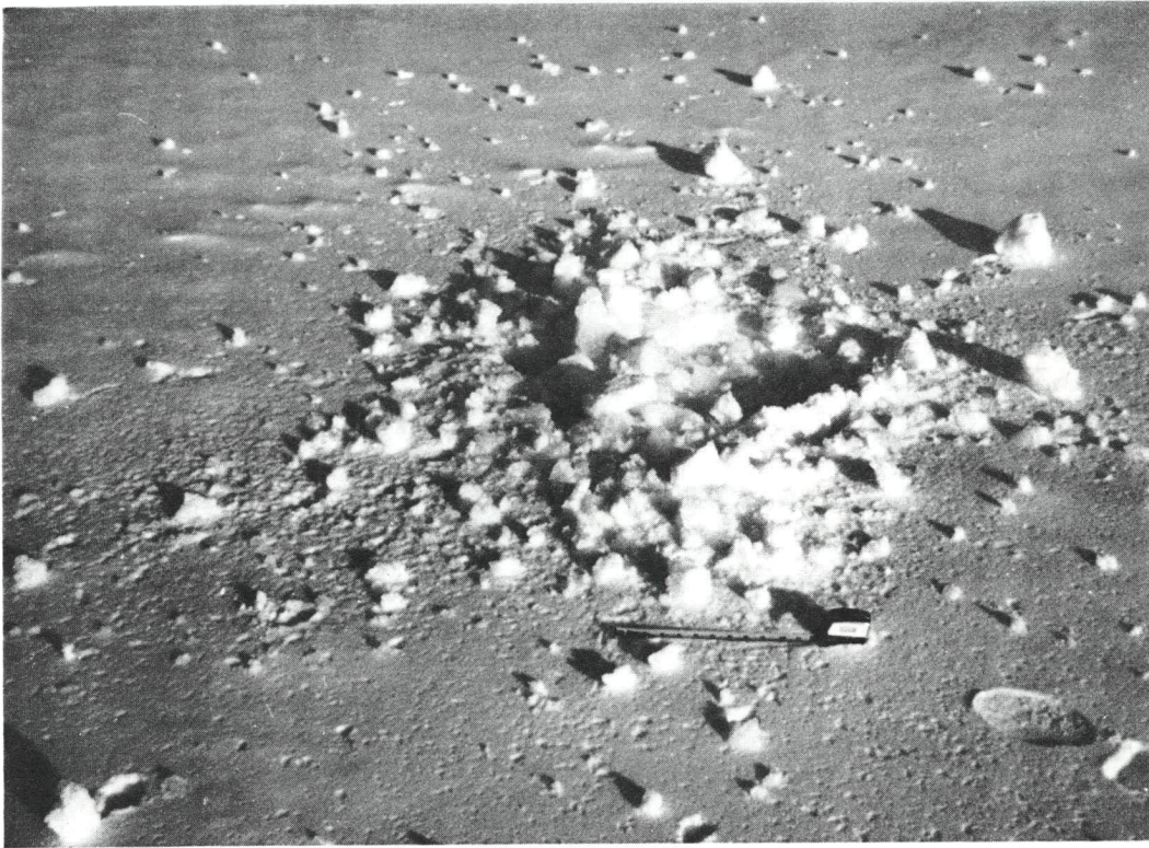
FIGURE 12 - Photographs of Ice Surface after Penetration
