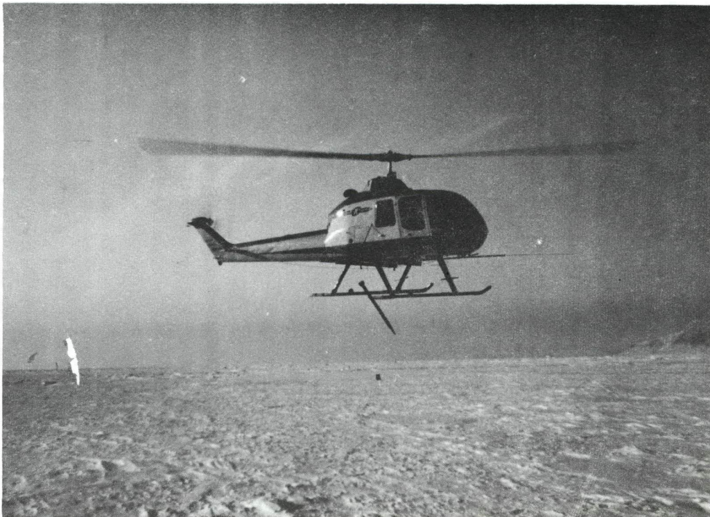
FIGURE 11 - Penetrator Slung under Helicopter Hovering over Target
