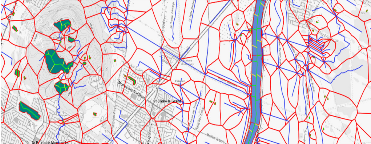
Figure 12: A catchment coverage (with boundaries rendered in red) extending across all of the terrain
