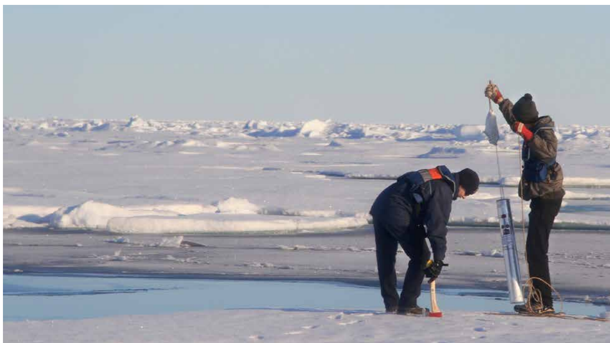
GSC scientists Patrick Meslin and Kai Boggild deploying a sonobuoy in the central Arctic Ocean, in the vicinity of the North Pole.
