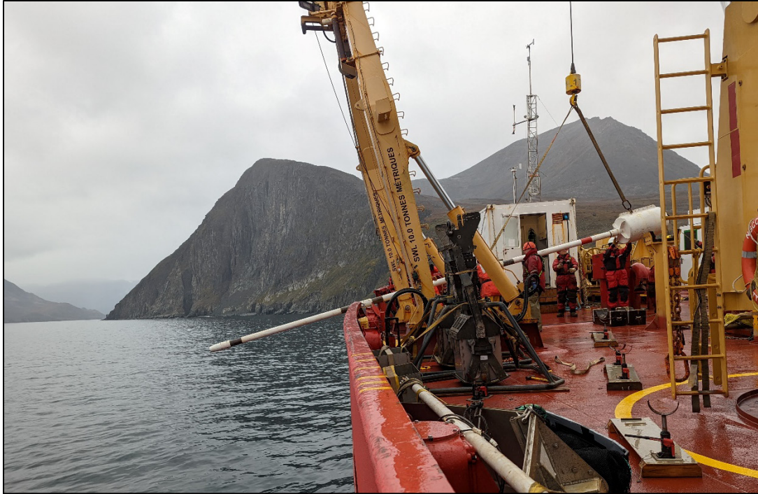
Figure 4: Gravity coring operations in Nachvak Fjord using the 9 m long core assembly. Photograph by L. Broom. NRCan photo 2023-050.
