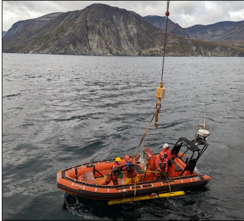
Figure 10: Retrieval of AUV using the CCGS Amundsen FRC. Photograph by L. Broom. NRCan photo 2023-054.
