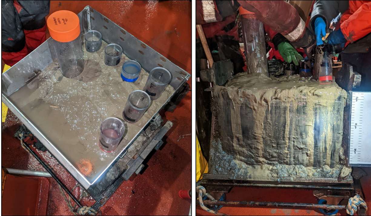
Figure 7: Box core collected from Nachvak Fjord, Labrador showing placement of push core (orange cap) collected by GSC-A. Photographs by L. Broom. NRCan photo 2023-051 and 2023-052.
