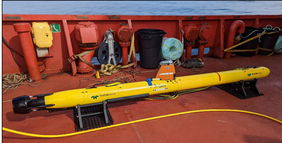
Figure 9: AUV used to collect high-resolution bathymetric data in Joey's Gully and Nachvak Fjord. Photograph by L. Broom. NRCan photo 2023-053.
