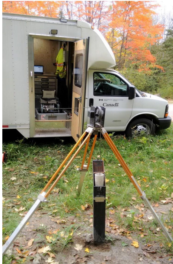
Figure 8. Typical geophysical logging set-up with the GSC's portable wireline logging system. Photograph by H. Crow. NRCan photo 2023-302.
