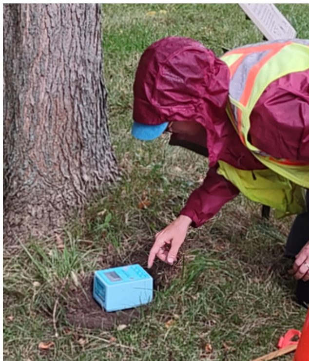
Figure 6. HVSR data collection. The digital seismograph is portable and designed for one-person use. To minimize the effects of wind and rain, a traffic pylon is commonly placed over the instrument. Photograph by H. Crow. NRCan photo 2023-300.
