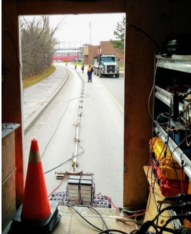
Figure 7. Reflection seismic acquisition in progress on Ian McDonald Road at the York University campus. The Microvibe, which produces and transmits the vibrations into the ground, is visible below the door opening of the acquisition van. The three-component geophones that record the reflected vibrations are mounted on sleds and pulled by a high-tension strap behind the Microvibe. Photograph by A. Pugin. NRCan photo 2023-301.
