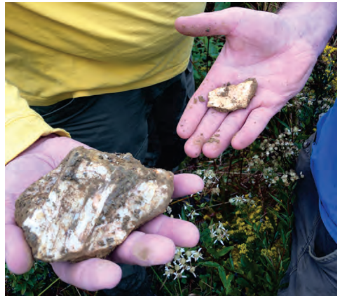
Figure 7. Spodumene clasts from the pegmatites were readily visible while sampling tills in backhoe trenches just down-ice of the pegmatites (photograph by M.B. McClenaghan, NRCan photo 2022-590).
