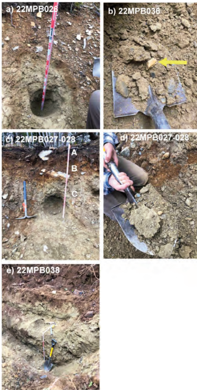
Figure 6. Examples of subglacial traction (lodgement) till sampled at various sites in the Brazil Lake study area. Note the compaction of the till as demonstrated by fissility and overconsolidation. Width of shovel head is 21 cm: a) site 22MPB026 after sampling; b) site 22MPB036, overconsolidated chunks of till on the shovel. Note the white spodumene clast indicated by the yellow arrow; c) site 22MPB027 after sampling showing well developed A, B, and C soil horizons; d) 22MPB027 overconsolidated chunk of till on shovel; e) site 22MPB-038 after sampling showing subhorizontal fissility behind the shovel. Photographs by M.B. McClenaghan, NRCan photo 2023-061, 2023-062, 2023-063, 2023-064, and 2023-065, respectively).
