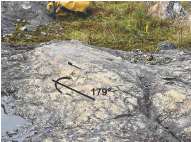
Figure 8. A striated bedrock surface that was exposed during previous stripping of the South pegmatite (photograph by D. Brushett, Nova Scotia Dept. Natural Resources and Renewables). The marker is 13.7 cm for scale.
