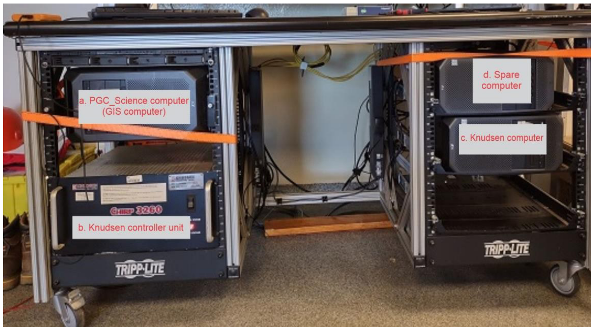
Fig. 1. NRCan Workstation. a. PGC_Science computer for collecting navigation data; b. Knudsen controller unit connecting the transducer; c. Knudsen computer for generating sub-bottom profiles; d. Spare computer. Photograph by R. Kung. NRCan photo 2023-324.
