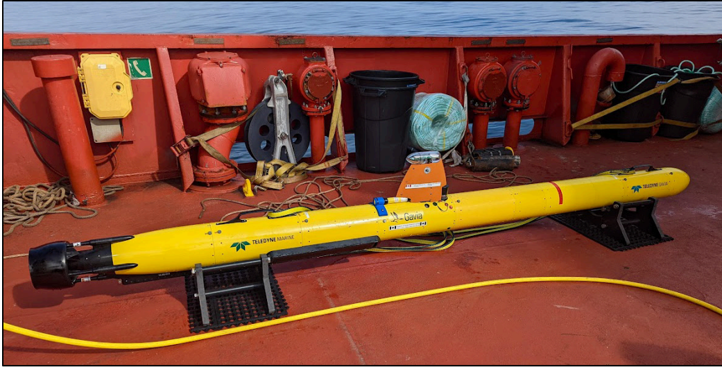
Figure 7: Photo of the Gavia AUV on deck. Photograph by L. Broom. NRCan photo 2023-053.
