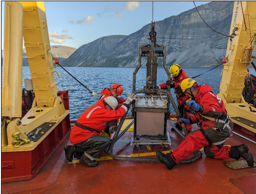
Figure 5: Deployment of the box core system in Saglek Fiord, Labrador Sea. Photograph by L. Broom. NRCan photo 2023-321.
