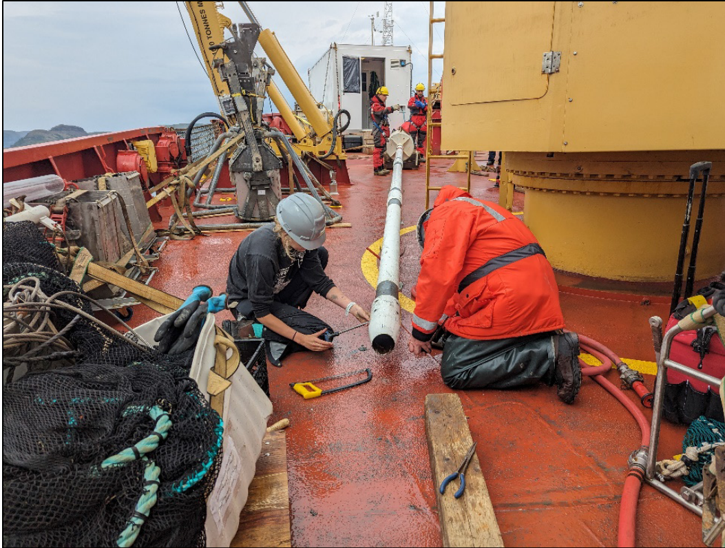
Figure 4: Image shows the gravity core system on deck and Margaret Atkinson (UNB) and Scott Hayward removing the core cutter from the bottom barrel. Photograph by L. Broom. NRCan photo 2023-320.
