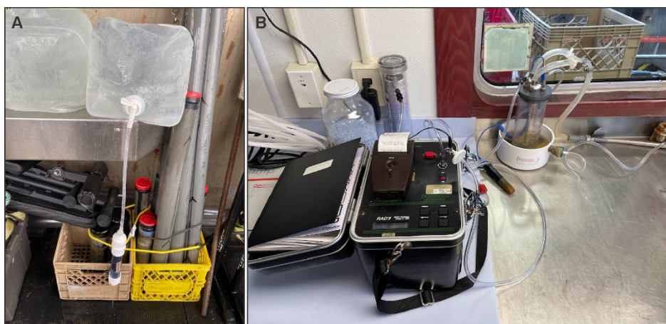
Figure 4. A) Gravity filtering for radium isotopes measurements and B) the RAD-7 setup. Courtesy of Jennifer Eamer.
