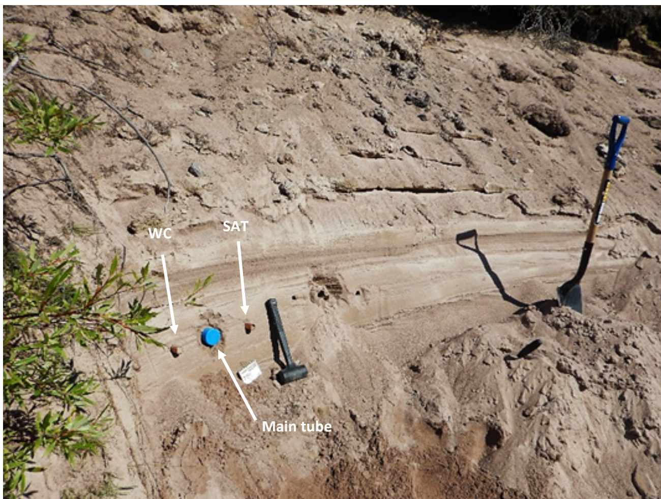
Figure 10. Example of an IRSL sampling site, photo 23BVB-B0015P018 (NRCan photo 2023-306). WC: Water content sample (copper tube). SAT: Saturation sample (copper tube).
