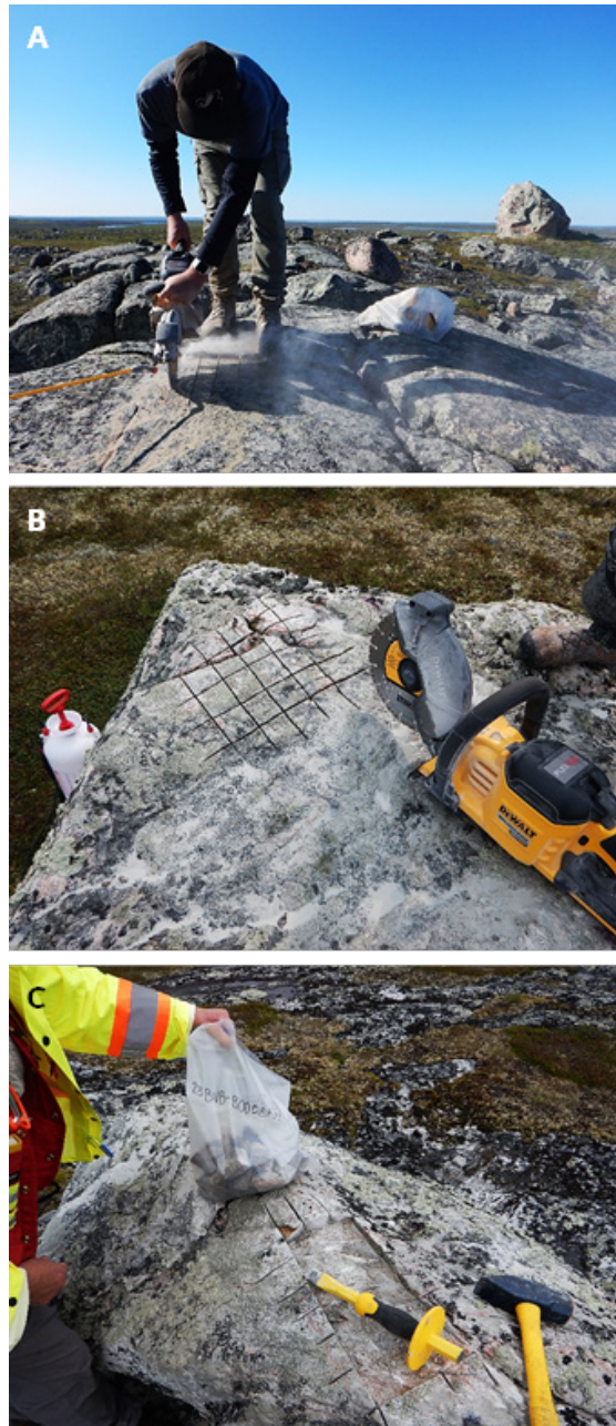
Figure 9. A. Example of TCN sampling using the portable rocksaw, photo 23BVB-B0025P002 (NRCan photo 2023-308). B. The resulting sampling grid, photo 23BVB-B0007P011 (NRCan photo 2023-304). C. Example of rock samples separated from the surface using a chisel and a hammer, photo 23BVB-B0008P007 (NRCan photo 2023-305).
