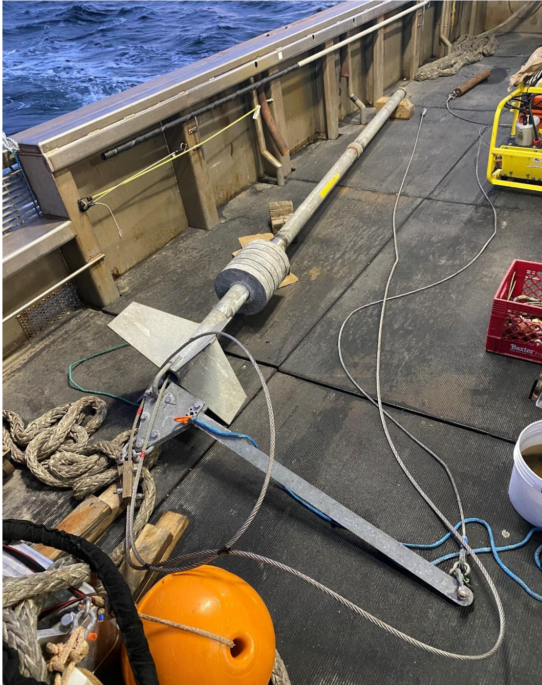
Figure 8. Mooring systems piston corer setup, including pilot weight in the top right and trigger arm in the foreground. The corer is the same as is used for a simpler gravity coring setup. Photograph by J.B.R Eamer. NRCan photo 2023-416
