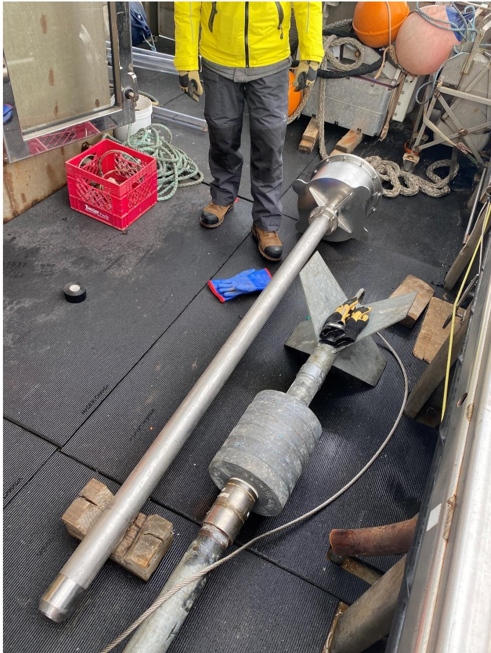
Figure 10. OSIL mini-vibrocoring (on left) and benthos gravity corer (on right). Photograph by J.B.R Eamer. NRCan photo 2023-418
