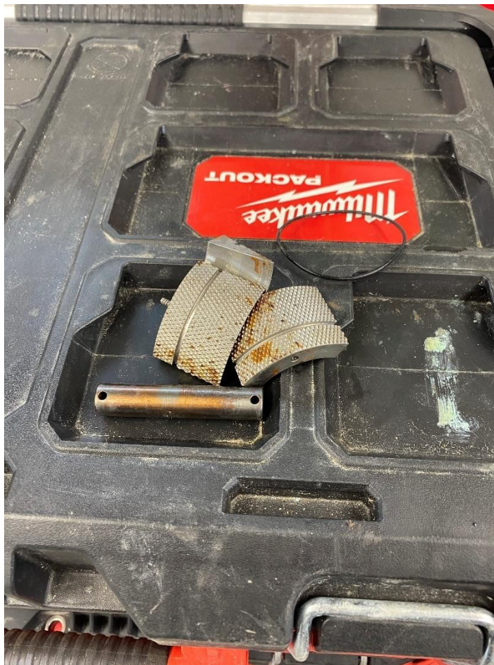
Figure 9. Pieces of the piston and pin recovered on deck. Photograph by J.B.R Eamer. NRCan photo 2023-417
