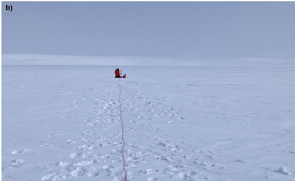
Figure 3. a) Schematic of TEM sounding survey layout (not to scale). b) View looking northeast towards the TEM receiver coil and operator at Site 1, Little Meliadine Lake, Nunavut. Photograph by K. Brewer. NRCan photo 2023-421.
