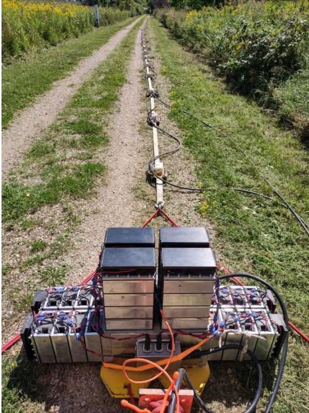
Figure 3. Microvibe and seismic landstreamer array being towed along the Elora Trail (Elora1). Photograph by H. Crow. NRCan photo 2023-299.
