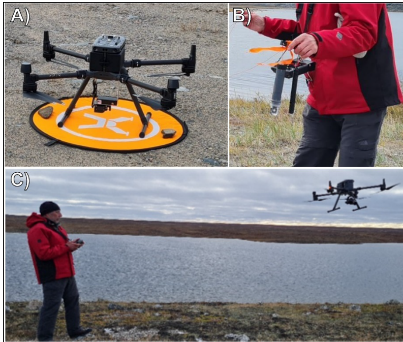
Figure 4: Photographs from the September 2023 field campaign showing A) a DJI Matrice 300 RTK Unmanned Aerial Vehicle (UAV) used for the depth profile surveys (photograph by É. Girard; NRCan photo 2023-518); B) the Solinst 5 LTC and HOBO MX2501 sondes attached to a 4mm thick Kevlar line attached to the UAV (photograph by É. Girard; NRCan photo 2023-519); and C) the UAV pilot flying the UAV during one of the lake physicochemical properties profile surveys (photograph by É. Girard; NRCan photo 2023-520).
