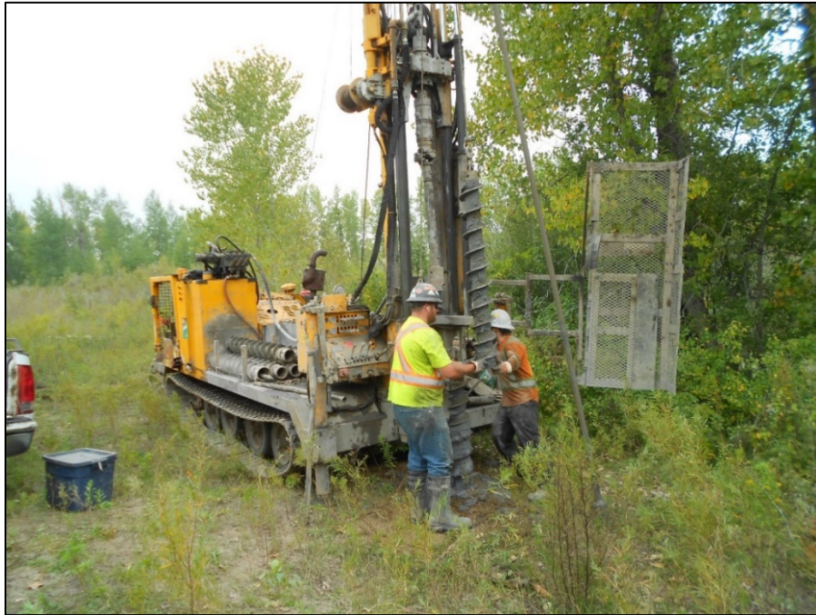
Figure 6: Drilling of the stratigraphic borehole by hollow-stem augering. Photograph by J.B. Percival. NRCan Photo Database number 2020-637.
