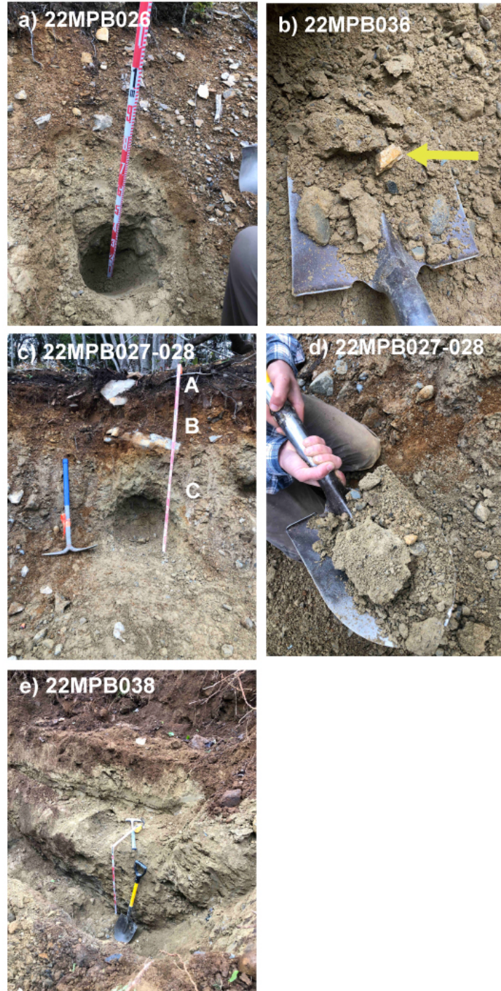
Figure 7. Examples of subglacial traction (lodgement) till sampled at various sites in the Brazil Lake area. Note the compaction of the till as demonstrated by fissility and overconsolidation. Width of shovel head is 21 cm: a) site 22MPB026 after sampling (photograph by M.B. McClenaghan, NRCan photo 2023-061); b) site 22MPB036, overconsolidated chunks of till on the shovel. Note the white spodumene clast indicated by the yellow arrow (photograph by M.B. McClenaghan, NRCan photo 2023-062); c) site 22MPB027 after sampling and showing well developed A, B, and C soil horizons (photograph by M.B. McClenaghan, NRCan photo 2023-063); d) 22MPB027 overconsolidated chunk of till on shovel (photograph by M.B. McClenaghan, NRCan photo 2023-064); and e) site 22MPB038 after sampling showing subhorizontal fissility behind the shovel (photograph by M.B. McClenaghan, NRCan photo 2023-065).
