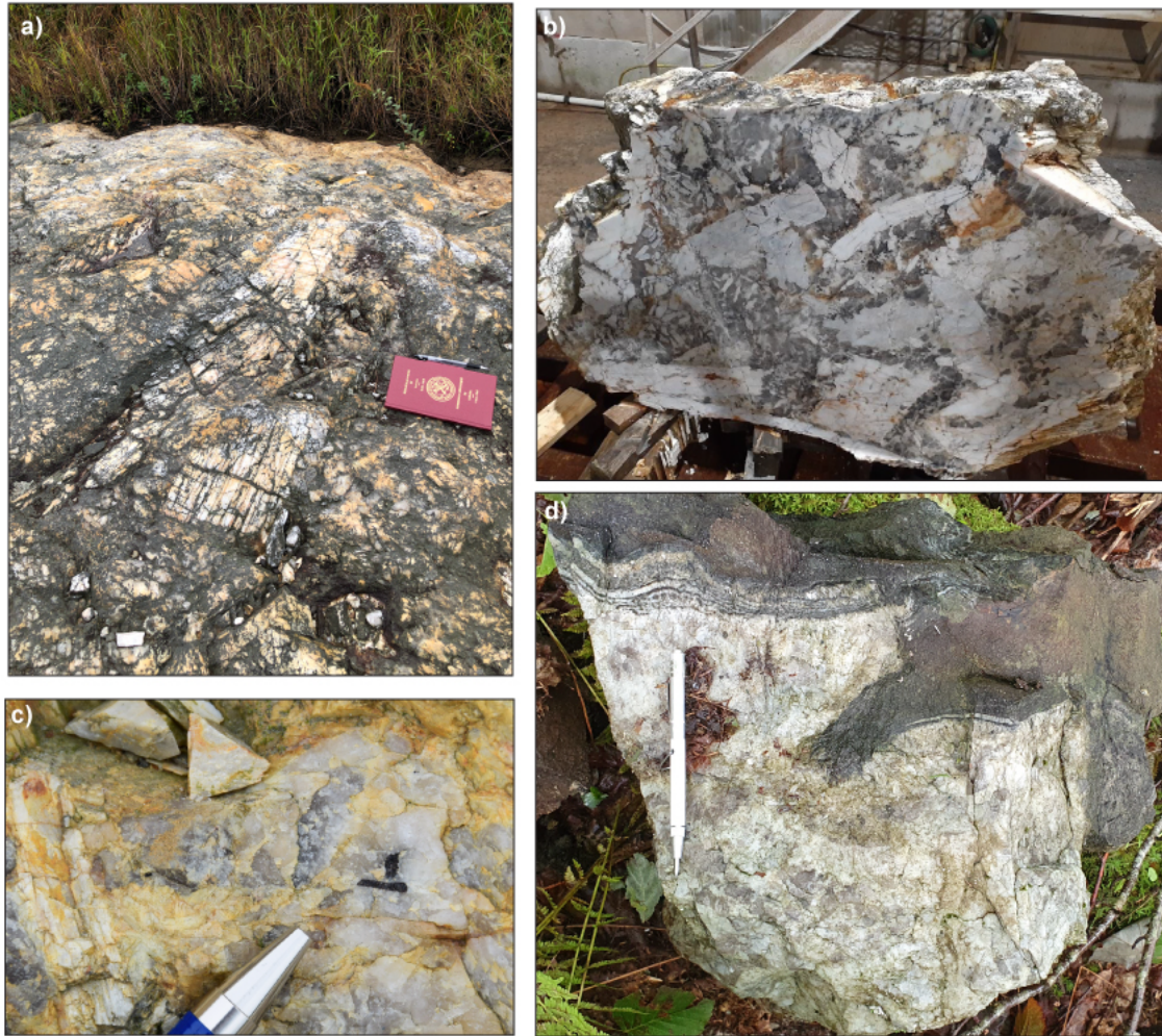
Figure 3. a) Coarse-grained ( \leq 0.5 m in length) white spodumene crystals exposed on the weathered subcropping surface of the South Dyke (photograph by M.B. McClenaghan; NRCan photo 2022-571); b) fresh unweathered spodumene boulder (1.5 m in length and 1.0 m in height) extracted from the South Dyke (photograph from Cullen et al., 2022); c) black columbite/tantalite crystals in quartz at the North Dyke (photograph by D. Archibald, St. Francis Xavier University); d) cross-section of the South Dyke in contact with the metavolcanic country rocks. At the outer contact of the pegmatite, abundant black tourmaline is observed, which formed as a result of the exsolution of boron-rich fluids from the pegmatite (photograph by C. Beckett-Brown; NRCan photo 2023-484).
