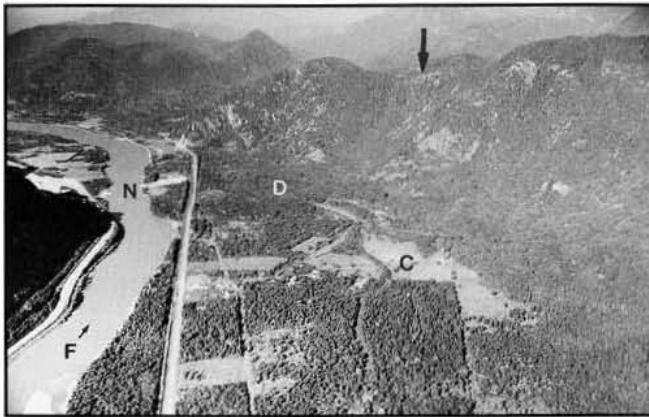
Figure 12. Oblique aerial view of Katz rock avalanche(s) looking southwest in the downstream direction of the Fraser River (F). The source area of the rock avalanche(s) is indicated with a vertical arrow. The debris in the Fraser Valley (D) blocked a channel of the Fraser River (C) and results in a constriction of the present Fraser River channel at point "N". (Photo by K.W. Savigny)
