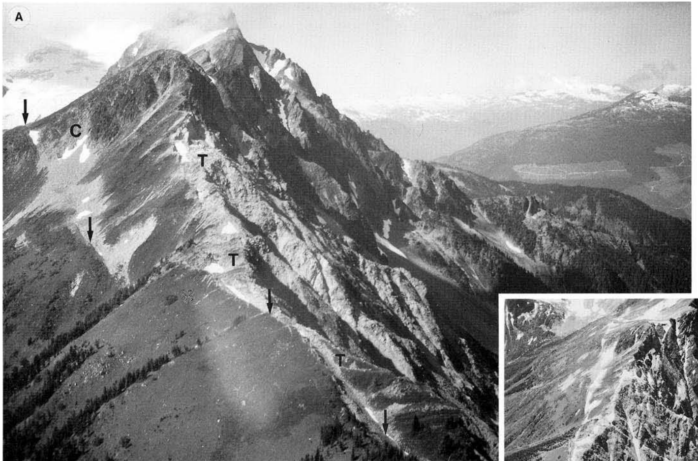
Figure 22. Slope deformation at Mount Currie, near Pemberton. A) Oblique aerial photograph of the northwest face of Mount Currie. Major linear discussed in text marked with vertical arrows. Also shown are areas of toppling (T), and the location of open cracks (C). GSC 204247-V. B) Oblique view of linears on summit ridge looking south-southwest along major linear. GSC 204045-V
