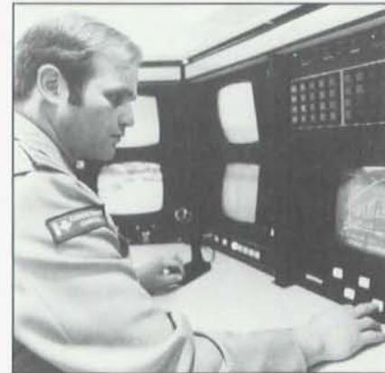
◀ Control panel of latest model of Perimeter Intrusion Detection System (PIDS) installed at Joyceville in late 1983.
