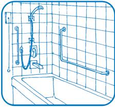
A bathtub with a non-slip surface and grab-bars, a hand-held shower with flexible tubing and a thermostatically controlled faucet will encourage independent use.
