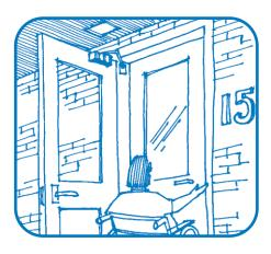
20 Storm doors are not recommended since they may create a problem to the user who would have to manage two doors at the same time. Storm doors can be removed or at least equipped with equalizers and adjustable low-pressure door closers. They should remain only if an enclosed porch or vestibule cannot be provided.
