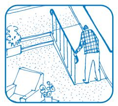
67 In areas with minor level changes (only a few steps), an **interior**ramp with a slope no steeper than 1:8 may be appropriate for wheelchair users or other persons with limiting disabilities.
