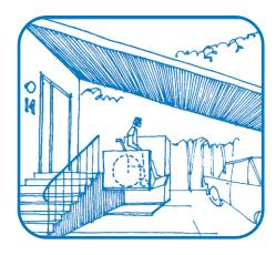
A chair lift could be considered if a ramp is not practical or desirable. If a chair lift is chosen, contact a local dealer for advice and estimates. Although porch lifts are generally weatherproof, they should be covered or fully enclosed so that they are operable in winter conditions.
