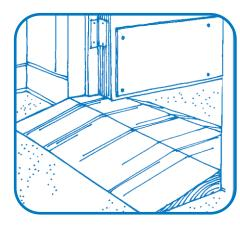
A **threshold** that is too high can be fitted with beveled strips.
