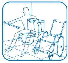
Extra free space on one side of the **toilet area** will allow a sideways transfer from a wheelchair. Grab-bars are needed to permit persons with disabilities to use the toilet independently. In some cases, a higher-than-standard toilet with built-in support rails or a commode chair for independent use may be an option.
