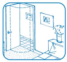
**94** Enlarged or sliding pocket doors will permit easier access, if space is limited.
