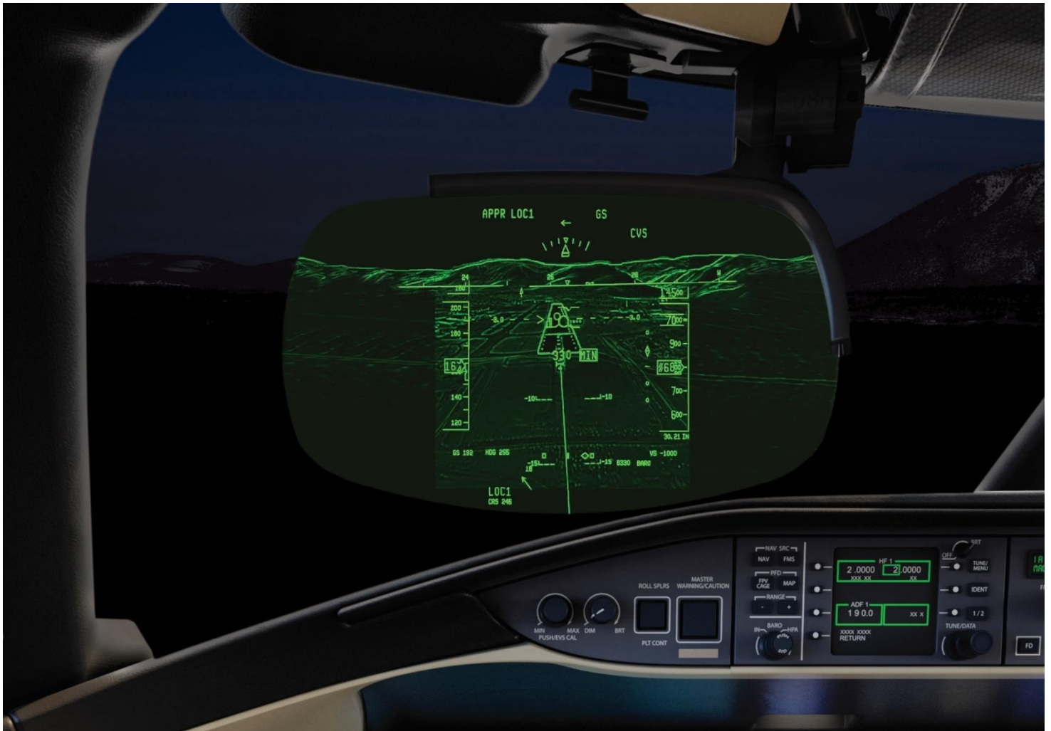
Figure 4: HUD system such as those which can be used for SA CAT I ILS approach procedures (Source: Bombardier Inc.).
