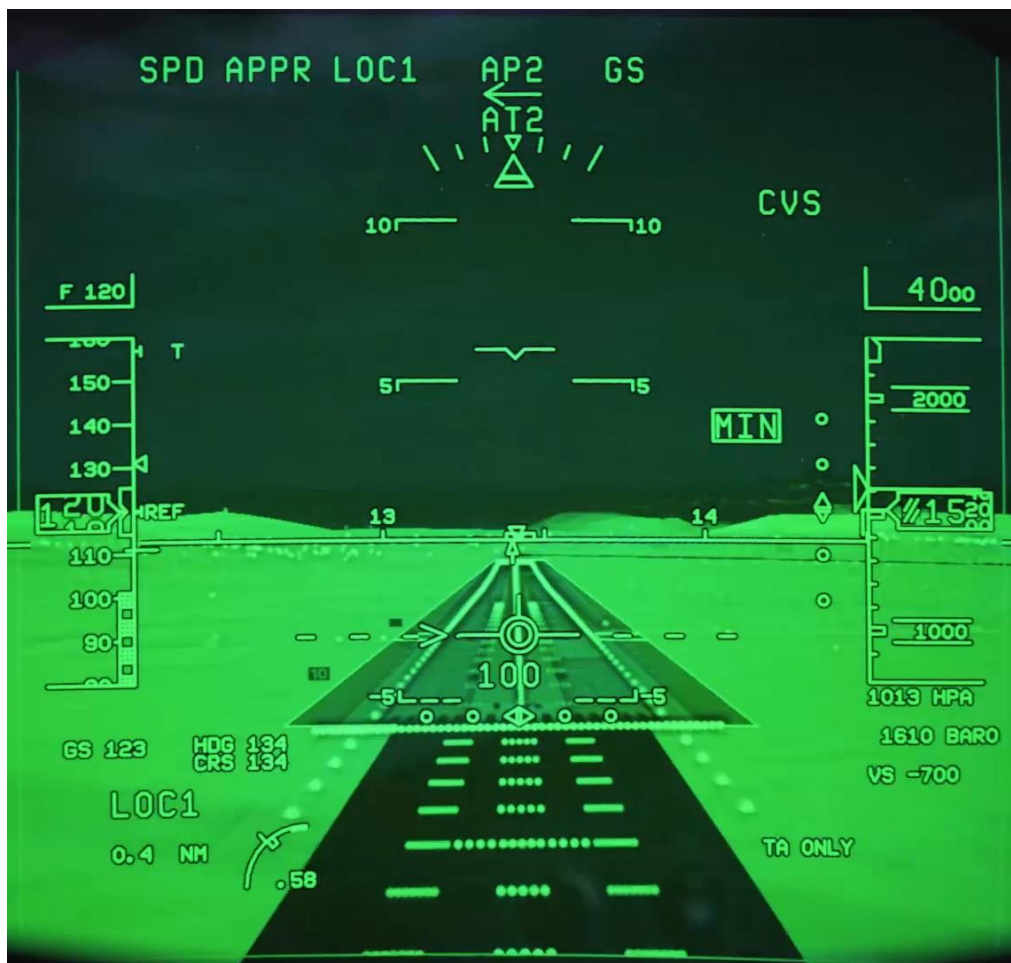
Figure 3: Combined vision system image which combines elements of EFVS and synthetic vision system (Proprietary to CAE Inc. © CAE Inc. 2024).
