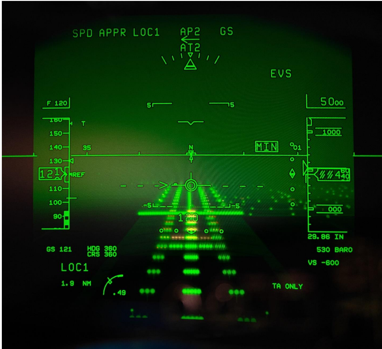
Figure 2: EFVS image displayed on an aeroplane's HUD (Proprietary to CAE Inc. © CAE Inc. 2024)
