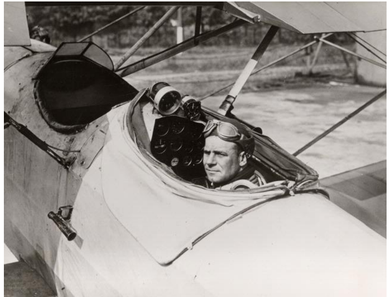
Lieutenant James H. Doolittle, Air Corps, United States Army, in rear cockpit of the Consolidated NY-2 Husky, NX7918, a trainer equipped with experimental flight instruments (Source: National Air and Space Museum, Smithsonian Institution (SI 79-9405)).
