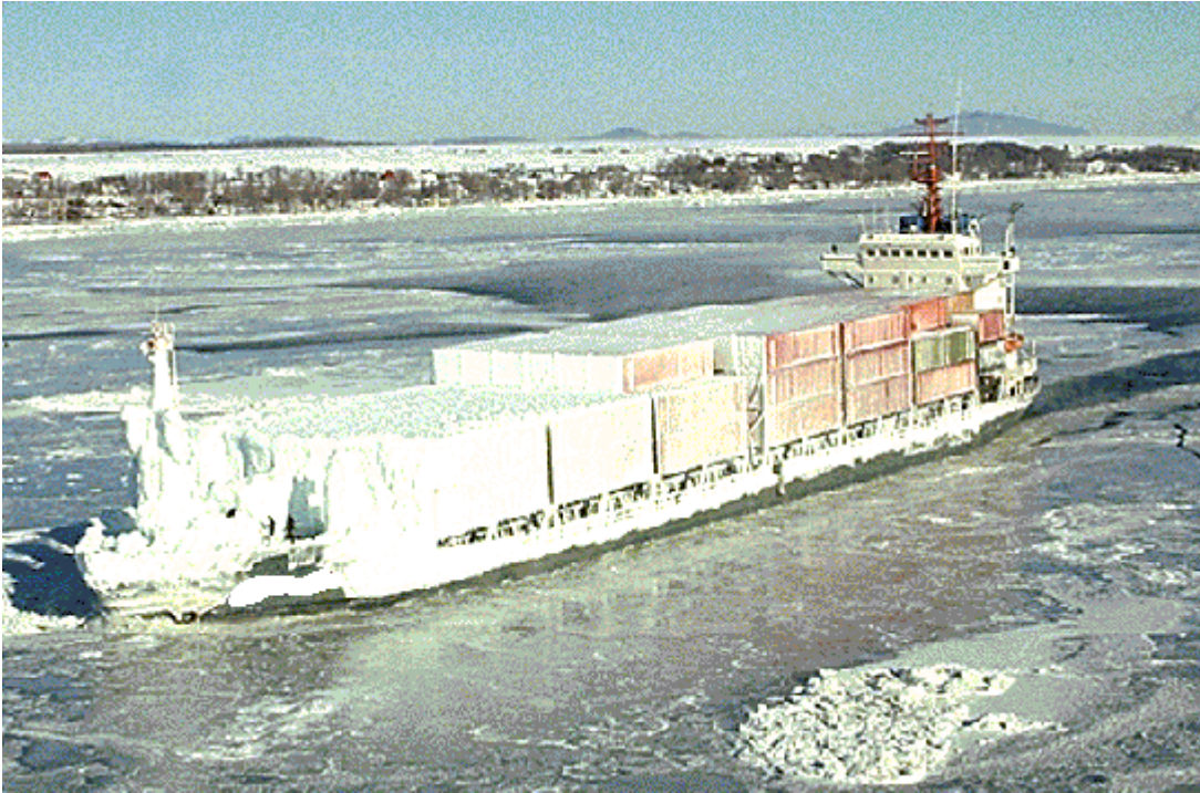
Figures 5.3M– Effect of freezing spray on a container ship
