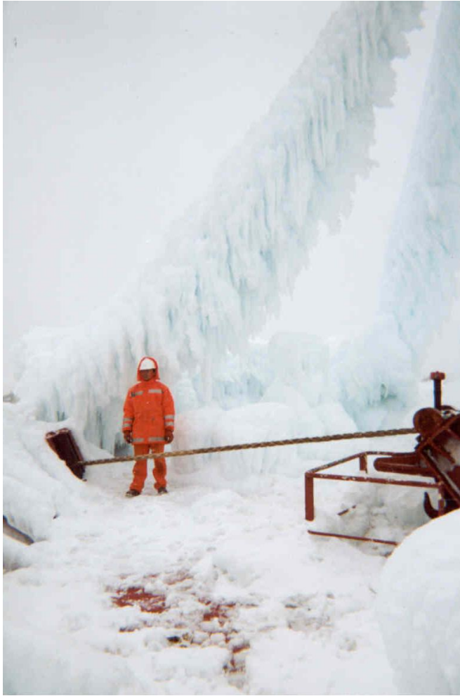
Figures 5.3G– Forward mast area guy wires draped in ice
