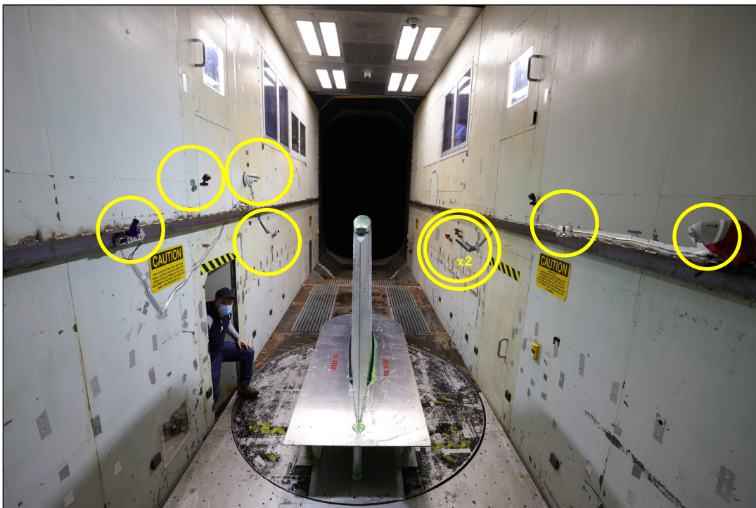
Photo 2.10: Location of Osmo® and CCTV Video Camera Mounts
