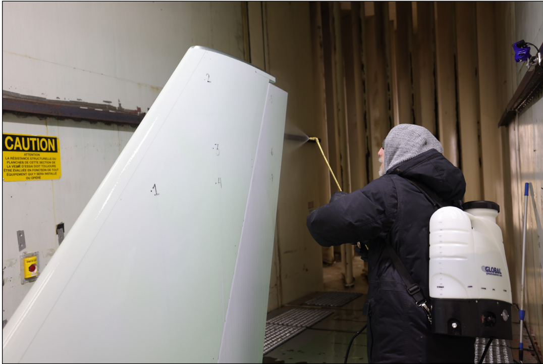
Photo 2.9: Simulating Freezing Rain with Garden Sprayer
