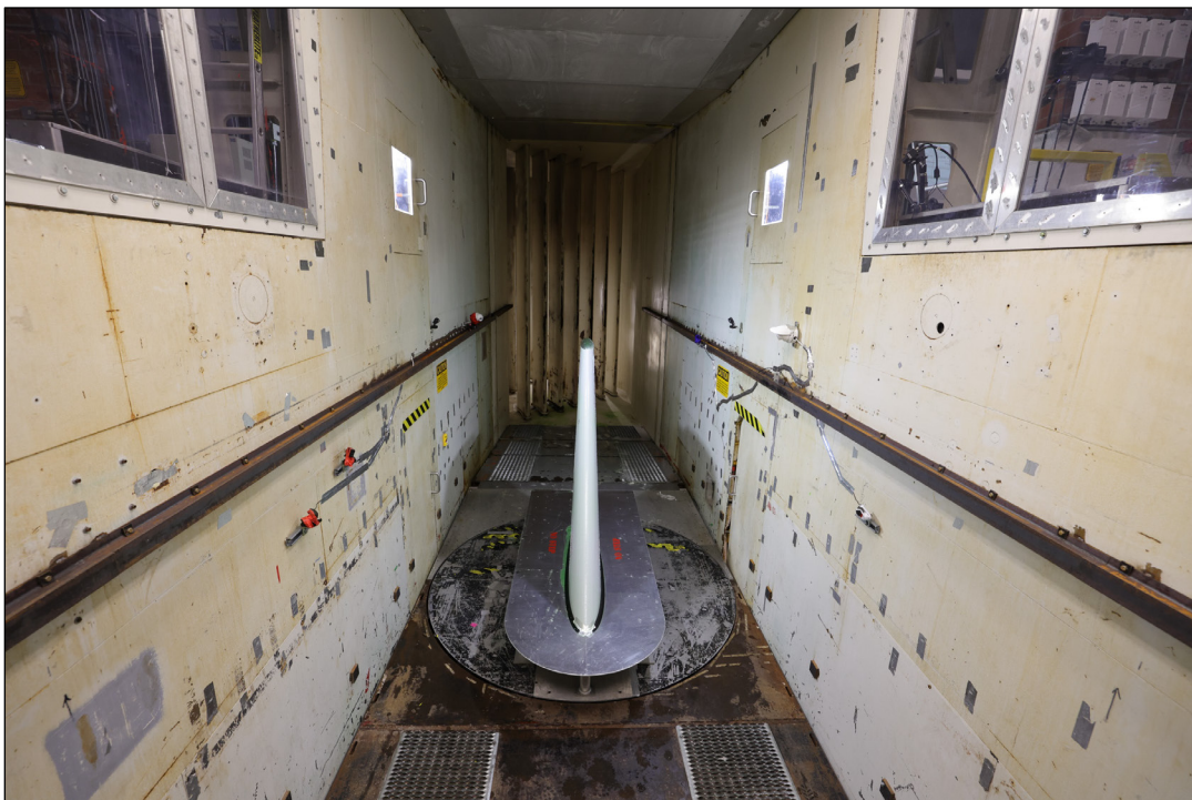
Photo 2.2: Inside View of the NRC Icing Wind Tunnel Test Section with the CRM
