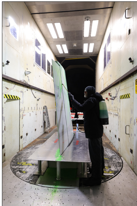
Photo 2.4: Vertical Stabilizer Mounted in the NRC IWT for Testing with Fluid Being Applied
