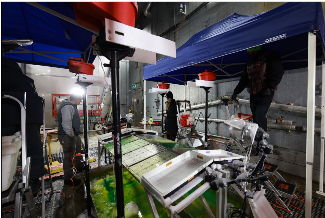
Photo 2.8: Mixed Conditions Test Stand with Rate Pans on Corner Positions
