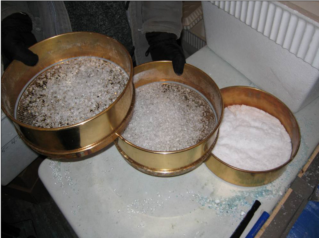
Photo 2.5: Calibrated Sieves Used to Obtain Desired Snow Size Distribution
