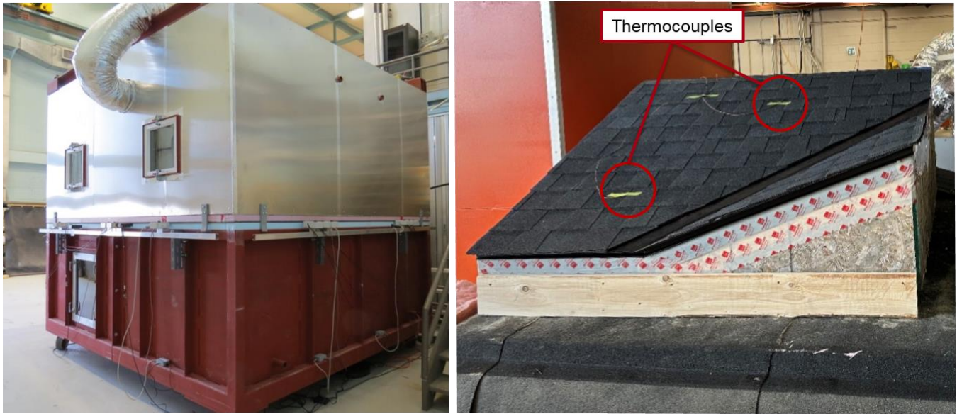
Figure 3. Environmental chamber to condition the test specimen
