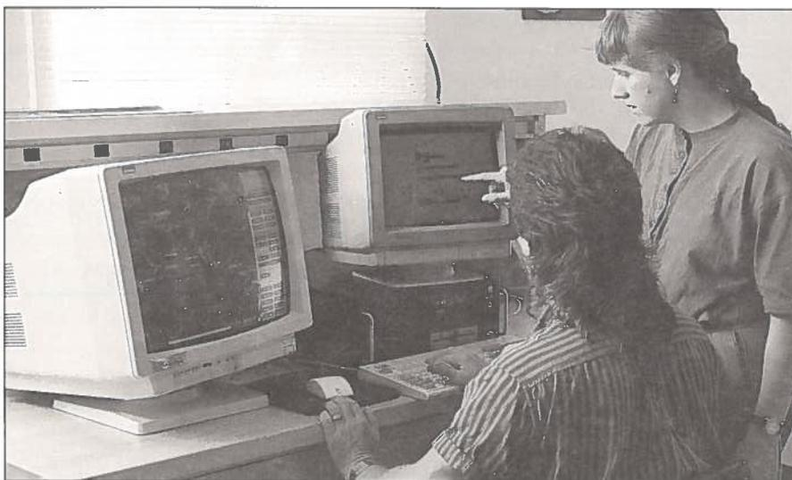
CRC Technologist Steve Lamarche and Engineer Trish Michaud operate Telesat Mobile's FLAG (Fleet Location and Graphics) dispatch base unit. The system was developed for MSAT to enable transportation companies to monitor the location of their vehicles. The unit in the picture is being used at the Communications Research Centre to give demonstrations and training sessions to potential users.
