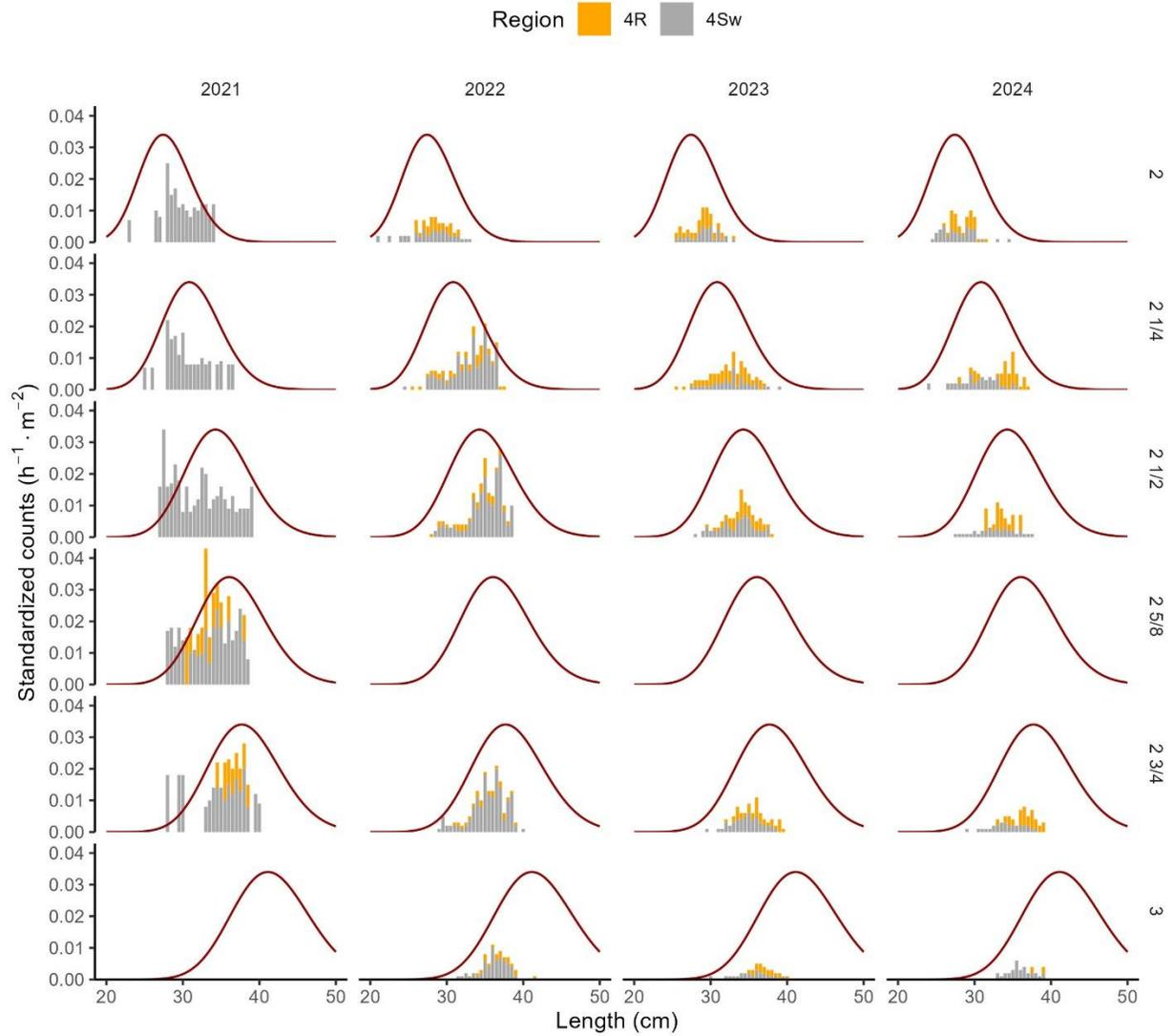
Figure 5: Standardized counts of fall spawning herring ( $\text{h}^{-1} \cdot \text{m}^{-2}$ ) caught per length class (cm), mesh size (inch; rows), year (columns) and region (colours). Data are used as input into the gillnet selectivity model. Red curves are estimated selectivity curves ( $\gamma$ ; see Table 3) scaled to the maximum observed counts.
