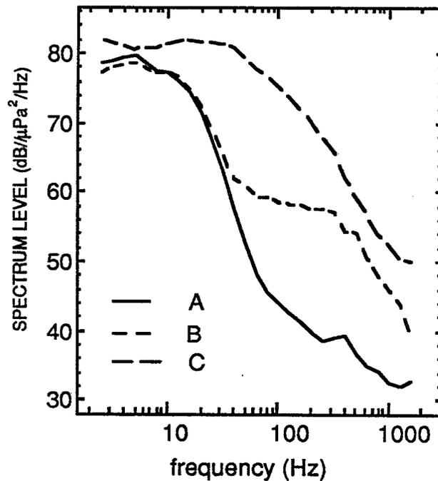
FIG.. 2. Noise spectrum level for the three ambient noise samples used for the present study. Sample A corresponds to a very quiet period, sample B contains thermal ice cracking, while sample C corresponds to a period of loud ambient noise caused by nearby lead formation.
