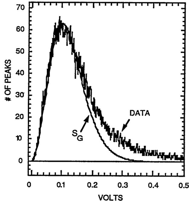
FIG. 1. Probability distribution function for the amplitude of the peaks in a Gaussian time series ( $S_G$ ) and measured histogram of the amplitude of peaks in a sample of ambient noise highpass filtered at 70 Hz.
