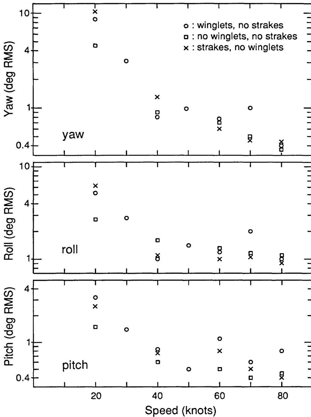
*Figure 7. The amplitudes of the 0.1-Hz pendulum motions deduced from the magnetometer signals applying the model described in the text. The amplitudes are accurate to ~20%.*
