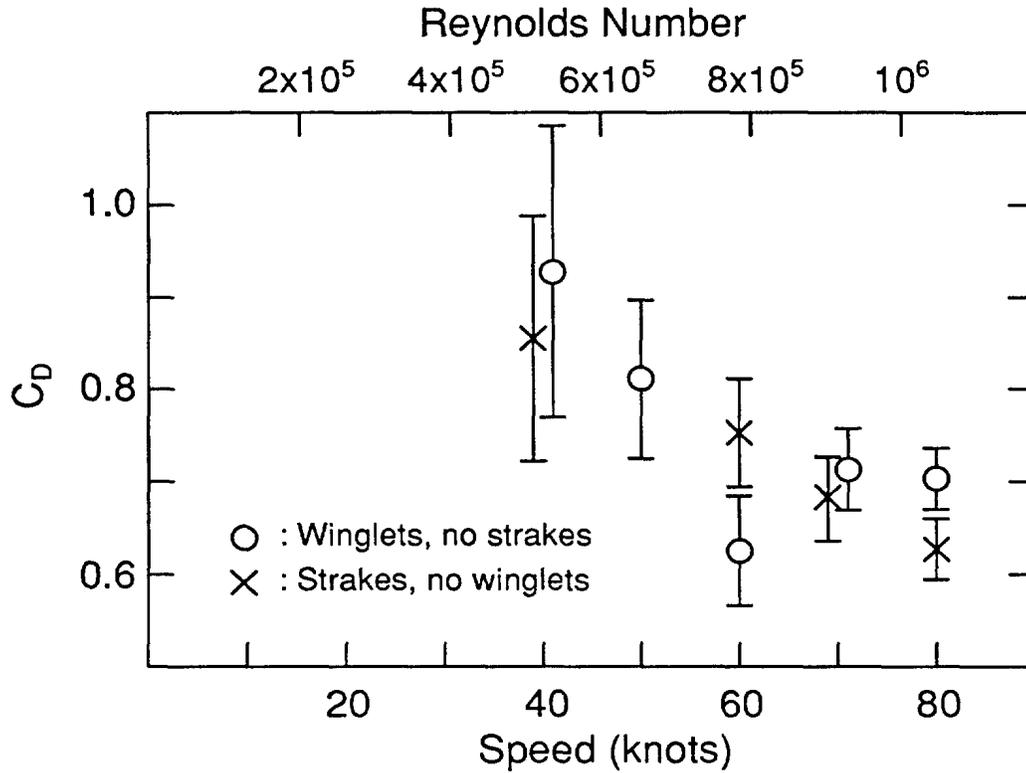
*Figure 6. The drag coefficient of the towbody deduced from the tow-rope angles.*
