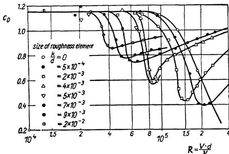
**Figure 2.** Drag coefficient for rough circular cylinders. (Ref. 2, Fig. 21.18).
