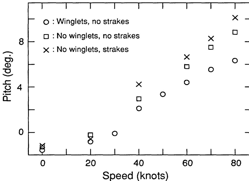
*Figure 5. Towbody pitch angle at speeds up to 80 knots measured by the 'forward' accelerometer.*
