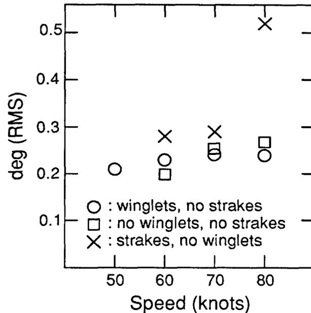
*Figure 10. RMS yaw amplitudes deduced from spectral analysis of the transverse and forward magnetometer signals.*
