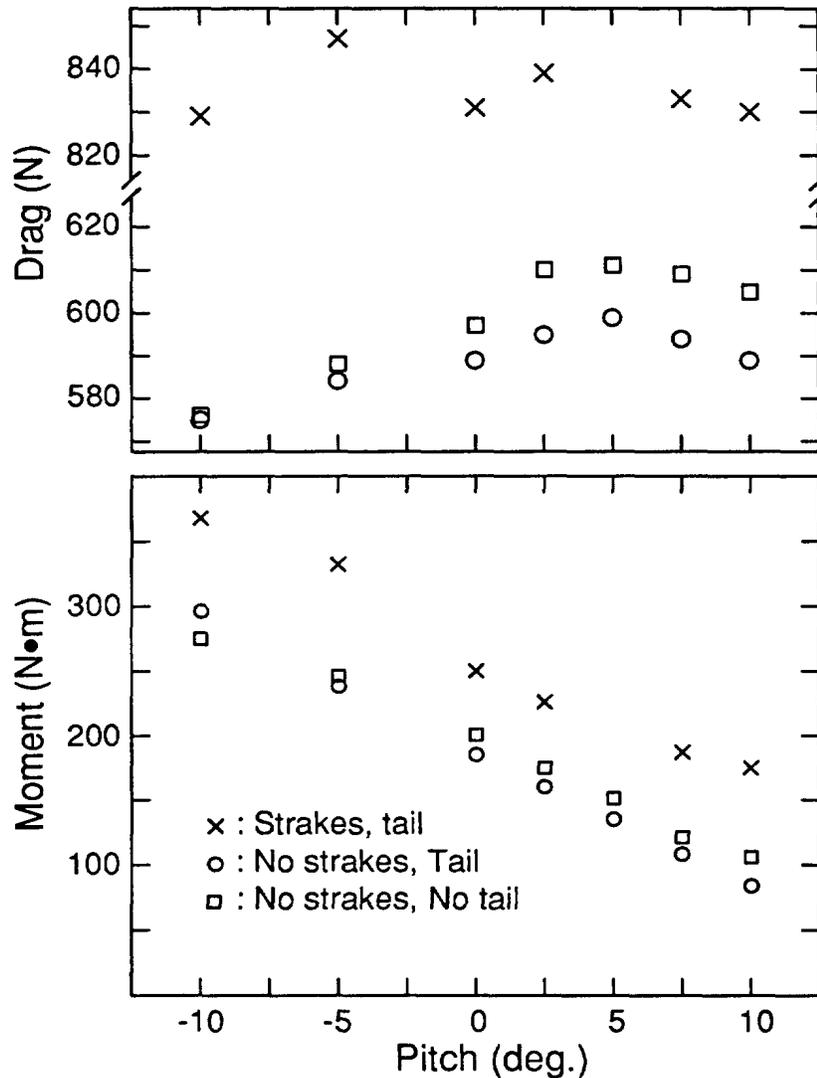
*Figure 3. Drag and pitching-moment measurements at 2.0 m/s water speed. Positive moment pitches the top of the towbody forward. No attempt has been made to correct systematic errors in the data.*
