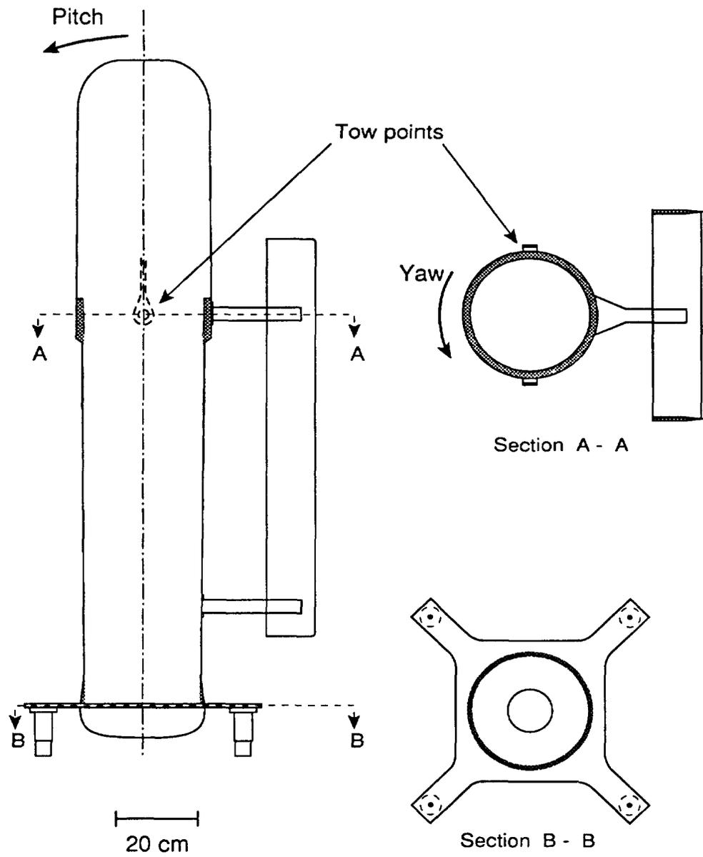
*Figure 1. An outline sketch of the towbody tested in the flight trials.*
