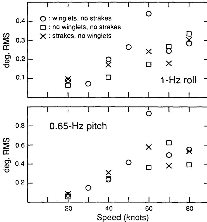
Figure 9. RMS roll and pitch amplitudes in straight and level flight derived from spectral analysis of magnetometer signals.
