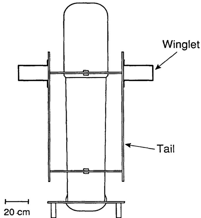
*Figure 4. Rear view of the towbody showing the winglets mounted on the tail.*
