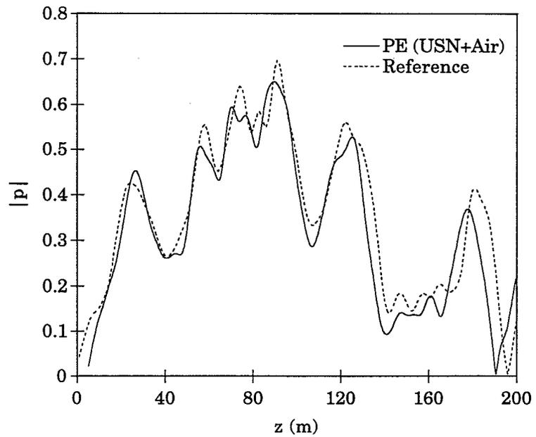
Fig. 8. US Navy standard PE (air-layer backing) versus reference solution.  $f = 400$  Hz.
