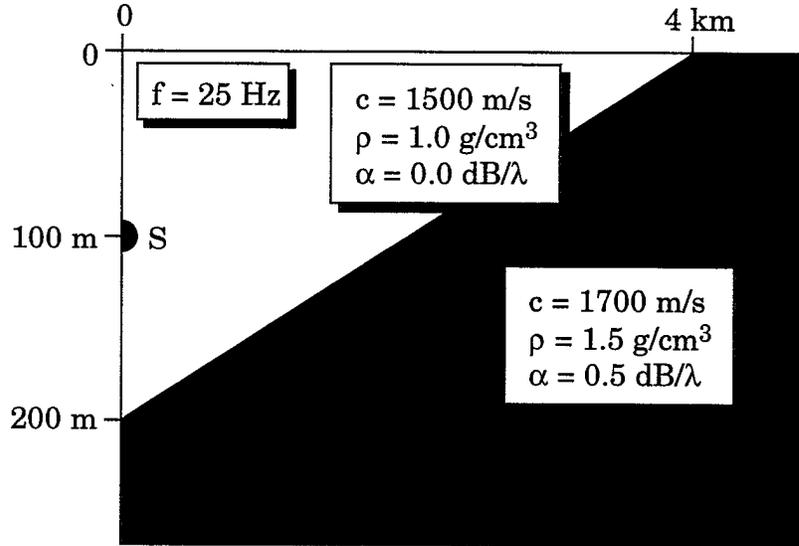
Fig. 13. Physical and environmental parameters for the ASA wedge.
