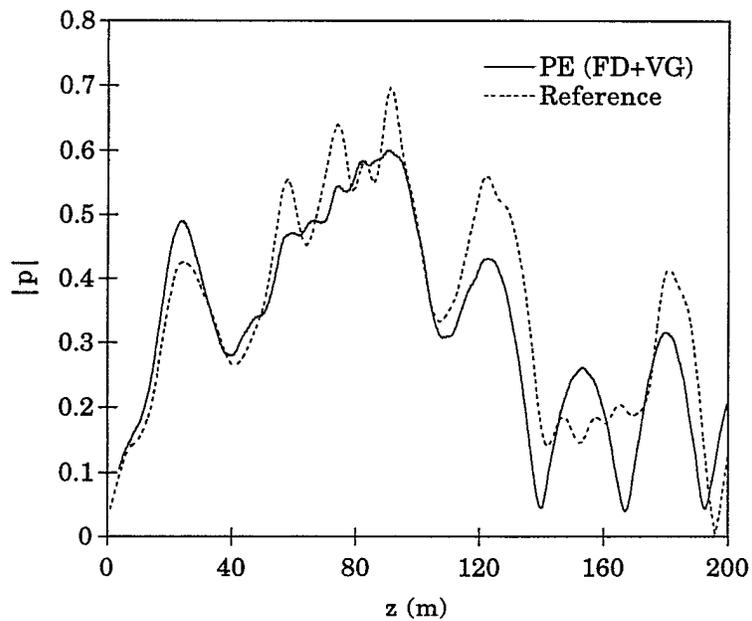
Fig. 4. Finite-difference PE (variable-depth grid) versus reference solution.  $f = 400$  Hz.
