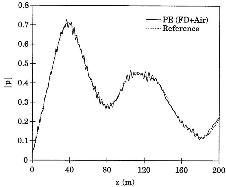
Fig. 5. Finite-difference PE (air-layer backing) versus reference solution.  $f = 100$  Hz.
