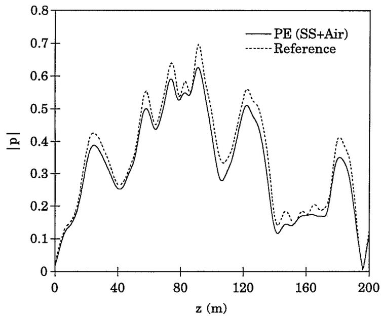
Fig. 12. Split-step PE (air-layer backing) versus reference solution.  $f = 400$  Hz.
