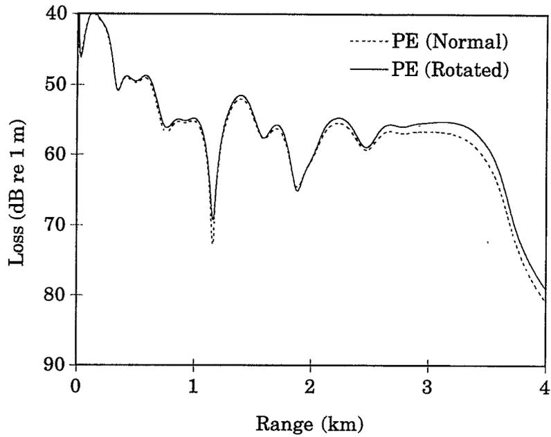
Fig. 15. Normal PE versus rotated PE solutions for the ASA wedge.  $z_r = 30$  m.
