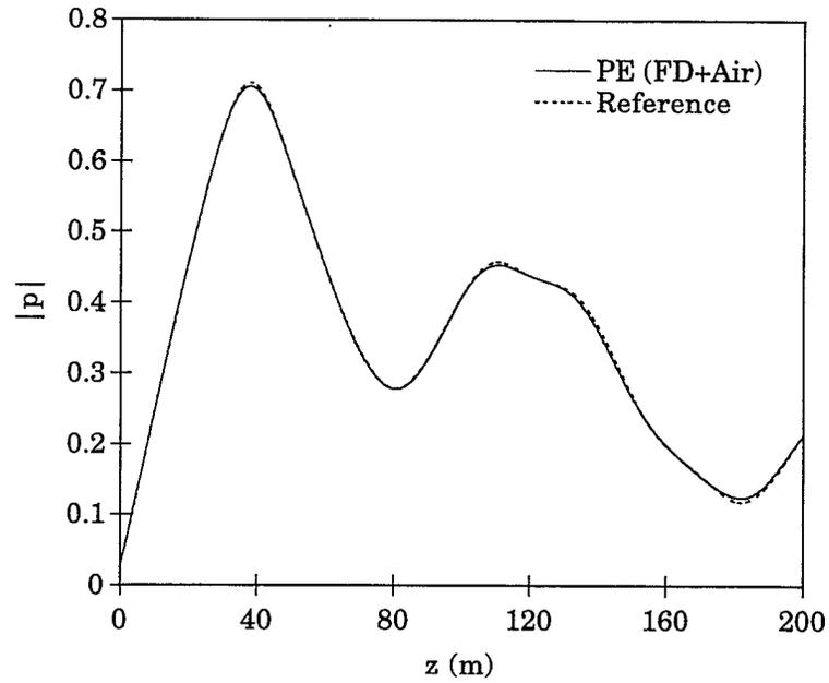
Fig. 9. Finite-difference PE (air-layer backing) versus reference solution.  $f = 100$  Hz.
