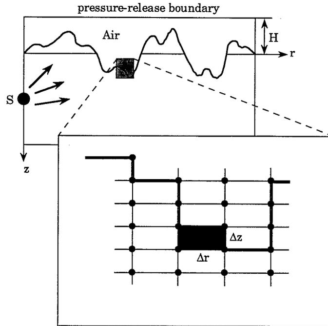
Fig. 2. Configuration for the air-layer backing method.
