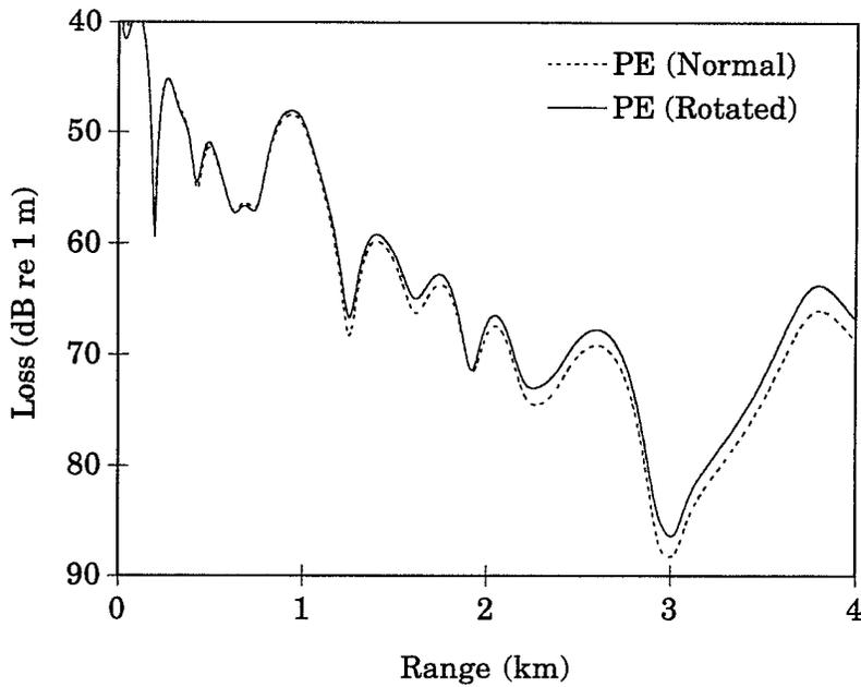
Fig. 16. Normal PE versus rotated PE solutions for the ASA wedge.  $z_r = 150$  m.
