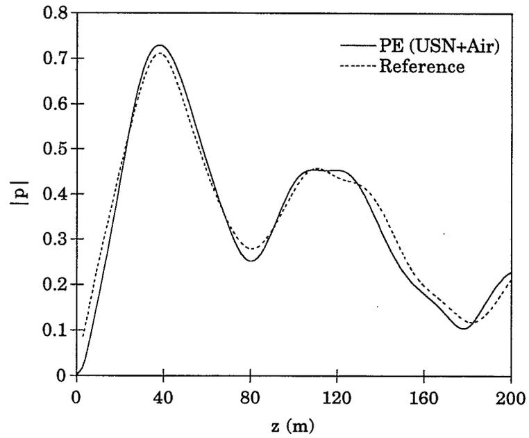
Fig. 7. US Navy standard PE (air-layer backing) versus reference solution.  $f = 100$  Hz.
