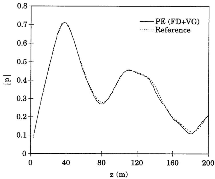
Fig. 3. Finite-difference PE (variable-depth grid) versus reference solution.  $f = 100$  Hz.
