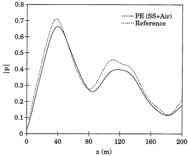
Fig. 11. Split-step PE (air-layer backing) versus reference solution.  $f = 100$  Hz.
