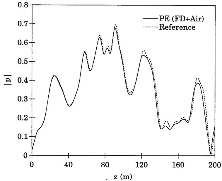
Fig. 10. Finite-difference PE (air-layer backing) versus reference solution.  $f = 400$  Hz.
