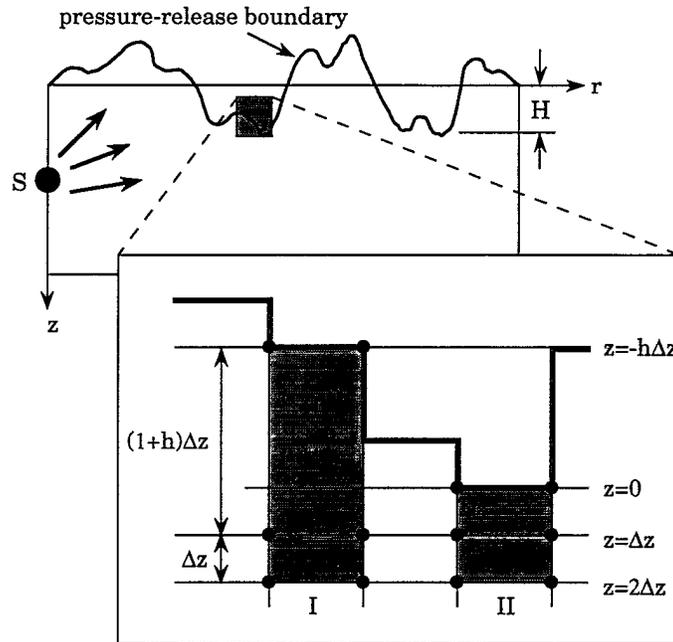
Fig. 1. Configuration for the variable-depth grid method.
