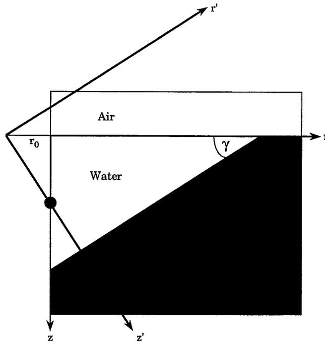
Fig. 14. Rotated coordinate system for the air-layer backed ASA wedge.
