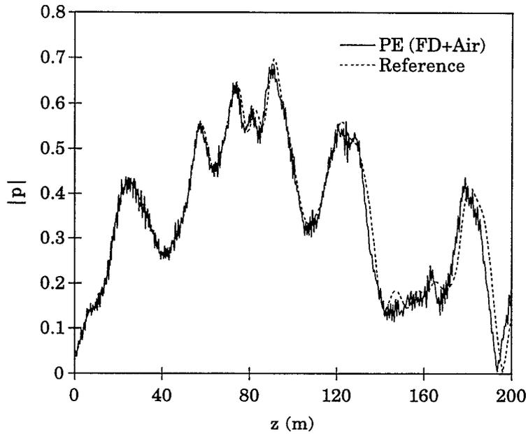
Fig. 6. Finite-difference PE (air-layer backing) versus reference solution.  $f = 400$  Hz.
