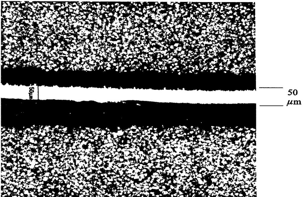
**Figure 22 Optical Micrographs of the Cross-Section of Lens C Showing Air Gaps Along the Dielectric/Adhesive Interface**
