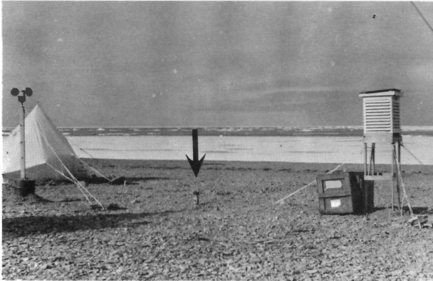
Figure 8.2. (A) Meteorological station located at the base camp, Cunningham Inlet (arrow locates rain gauge). (GSC 169681)
