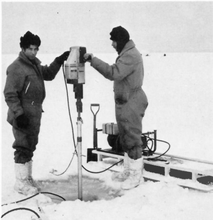
Figure 2.3 Sediment coring operation. Portable 3 Kw used to drive the hammer is partially visible on the back of the sled.
