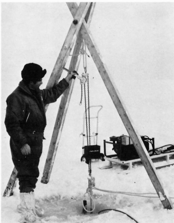
Figure 2.4 Core extraction hardware. Chain hoist is attached directly to the core head using a suitable rope which must be retied after each 0.6 m pull.
