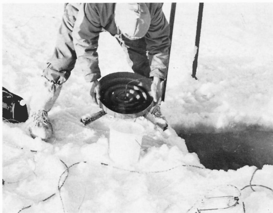
Figure 1.3. Decanting sediment slurry from the sediment bottle. Residual sediment was washed free using a dilute solution of standard automotive antifreeze.
