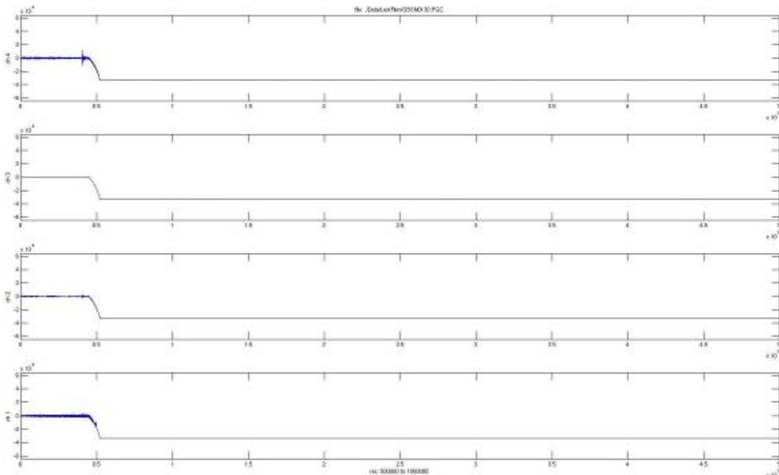
**Figure 9d.** End of recording cycle on OBS #4, NRCan-N, from regional grid. Horizontal axis is sample-number (sampling rate is 500 Hz, total record length shown is 1000 seconds). All four channels are shown (ch1: hydrophone; ch2: vertical; ch3=horizontal 1; ch4: horizontal 2).
