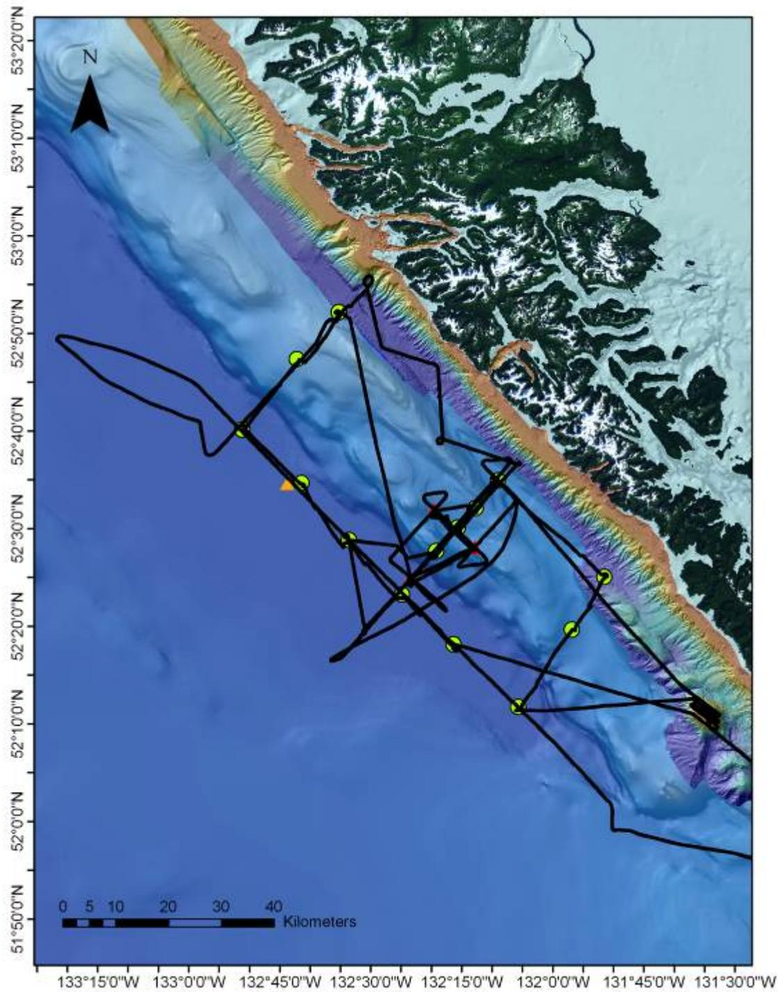
**Figure 3a.** All lines run during expedition. OBS locations from regional grid (green circles) and 2<sup>nd</sup> refraction experiment (red triangles) are shown, as well as the ODAS mooring site (orange triangle).
