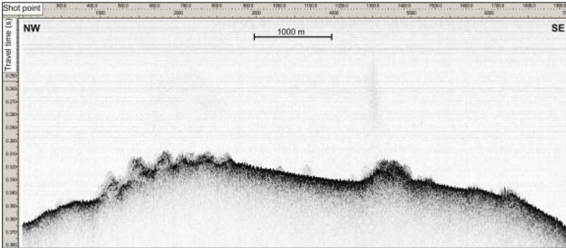
**Figure 7.** Example of the 3.5 kHz data recorded across plateau-feature on the last day returning to Port Hardy. Individual knoll-features produce chaotic signal from surface roughness. Note the hint of the gas plume at the largest knoll feature, near shot point 1300.
