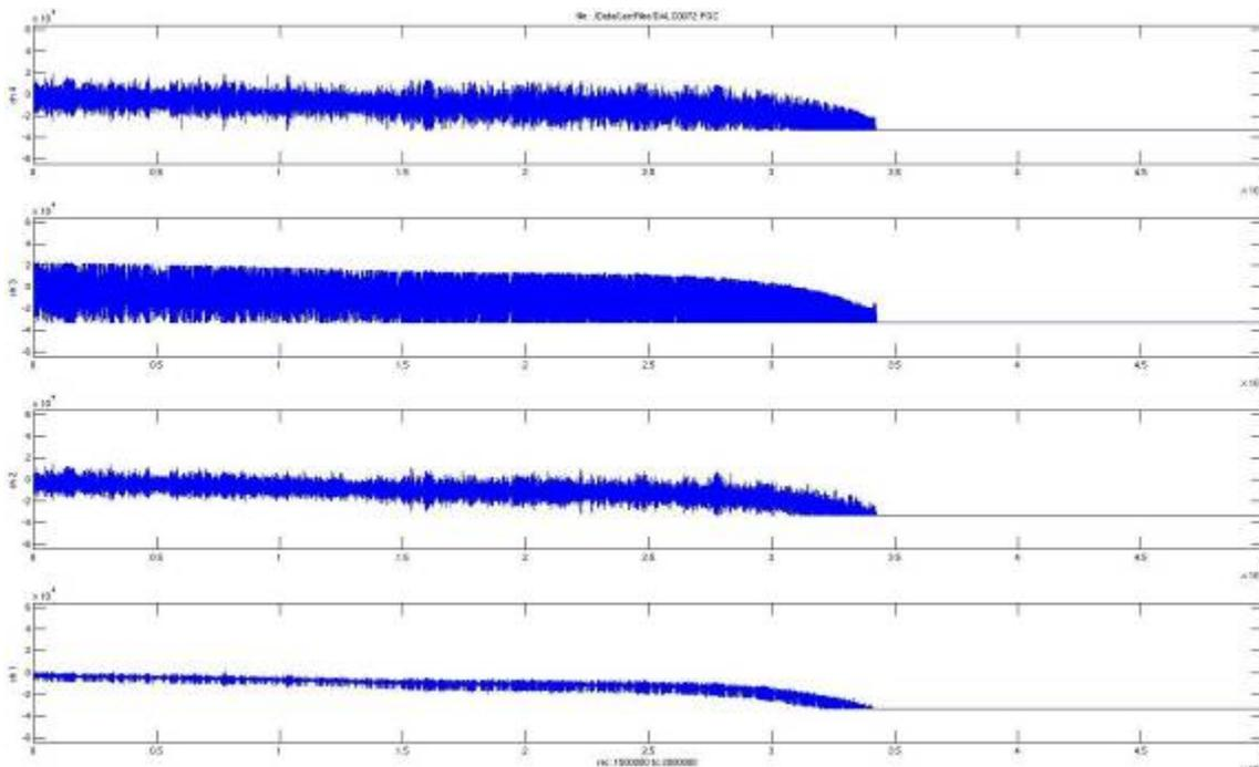
**Figure 9n.** End of recording cycle on OBS #14, Dal-C, from regional grid. Horizontal axis is sample-number (sampling rate is 500 Hz, total record length shown is 1000 seconds). All four channels are shown (ch1: hydrophone; ch2: vertical; ch3=horizontal 1; ch4: horizontal 2).
