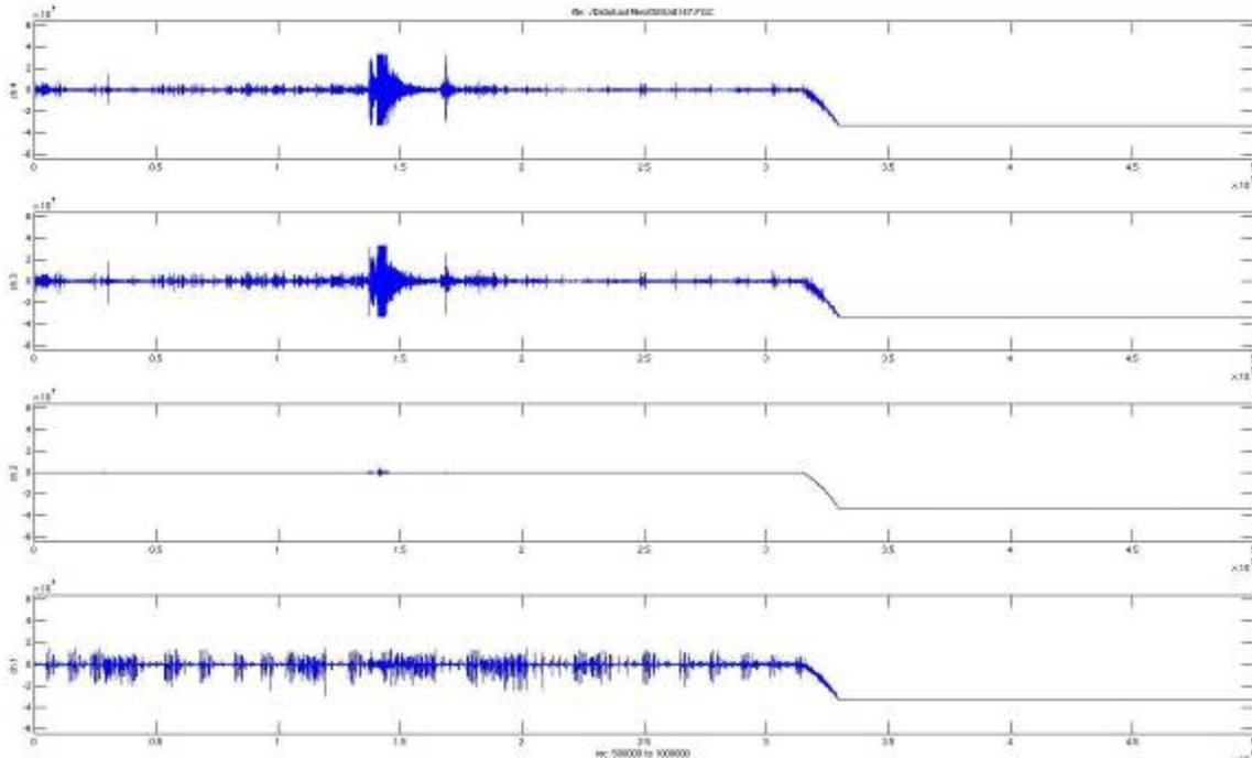
**Figure 9m.** End of recording cycle on OBS #13, NRCan-A, from regional grid. Horizontal axis is sample-number (sampling rate is 500 Hz, total record length shown is 1000 seconds). All four channels are shown (ch1: hydrophone; ch2: vertical; ch3=horizontal 1; ch4: horizontal 2).
