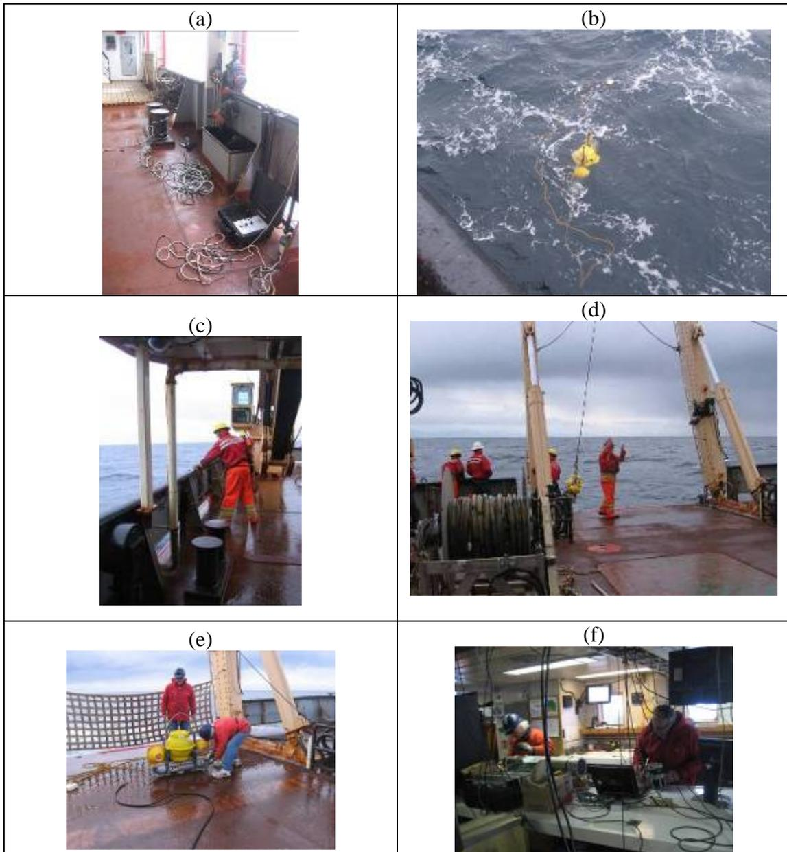
**Figure 4.** Sequence of OBS recovery: (a) installation of acoustic pinger and hydrophone for OBS release operation on starboard breezeway of the *CGGS John P. Tully*, (b) Floating OBS with rope attached, (c) Coast Guard personnel ready to through grappling iron to catch rope, (d) OBS secured with second rope, lifted onboard with A-frame and central winch, (e) OBS secured on deck, ready to be dismantled by scientists, (f) OBS pressure case inside dry-lab for data recovery.
