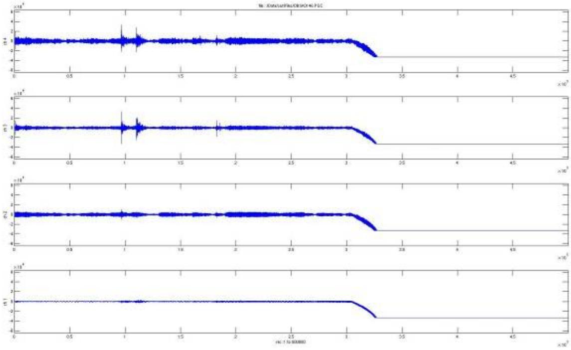
**Figure 9a.** End of recording cycle on OBS #1, NRCan-K, from regional grid. Horizontal axis is sample-number (sampling rate is 500 Hz, total record length shown is 1000 seconds). All four channels are shown (ch1: hydrophone; ch2: vertical; ch3=horizontal 1; ch4: horizontal 2).
