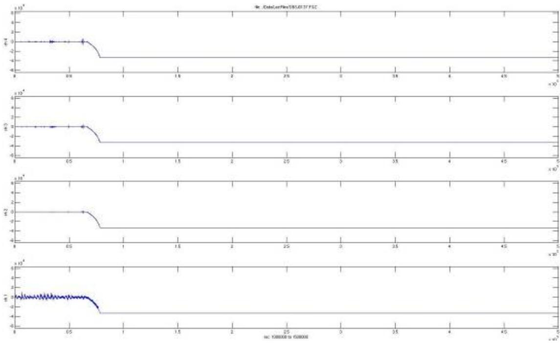
**Figure 9b.** End of recording cycle on OBS #2, NRCan-J, from regional grid. Horizontal axis is sample-number (sampling rate is 500 Hz, total record length shown is 1000 seconds). All four channels are shown (ch1: hydrophone; ch2: vertical; ch3=horizontal 1; ch4: horizontal 2).
