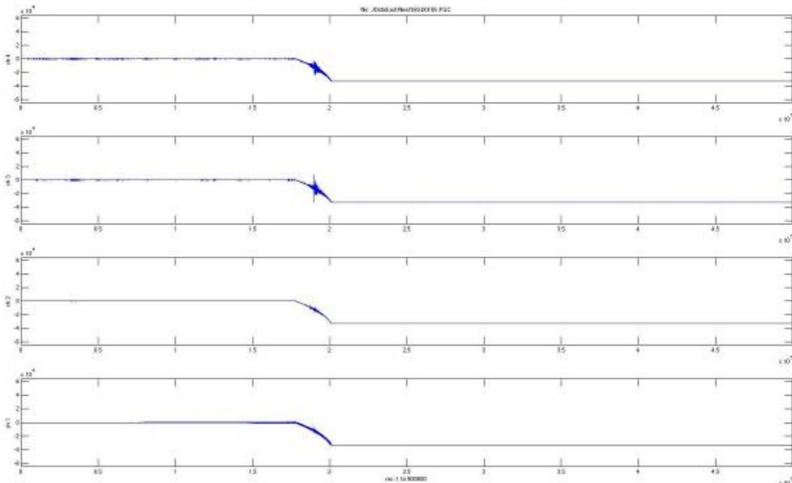
**Figure 9l.** End of recording cycle on OBS #12, NRCan-D, from regional grid. Horizontal axis is sample-number (sampling rate is 500 Hz, total record length shown is 1000 seconds). All four channels are shown (ch1: hydrophone; ch2: vertical; ch3=horizontal 1; ch4: horizontal 2).
