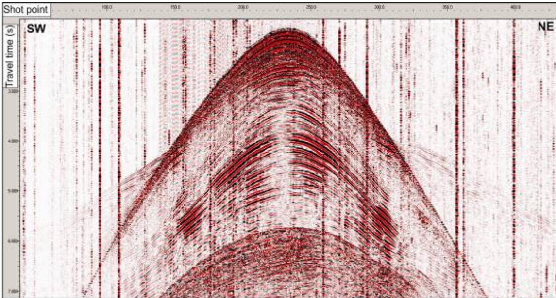
**Figure 6.** Example of airgun data recorded on D2 OBS #6 (western-most station of second refraction experiment) showing portion of SW-NE-trending main central line shot upslope across the terrace region. Clear refractions can be seen on both side of the shot-record.
