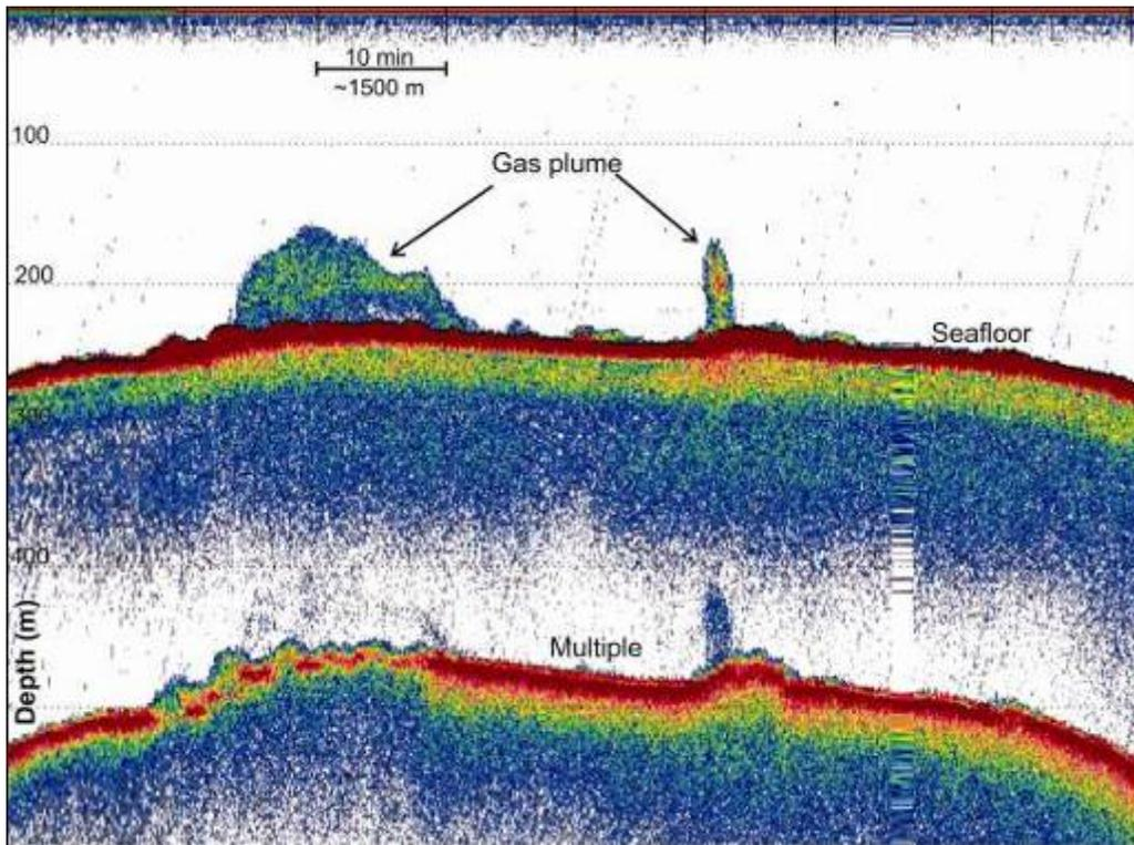
**Figure 8.** Example of the 12 kHz data recorded across plateau-feature on the last day returning to Port Hardy. Two large gas plumes are evident in the record.
