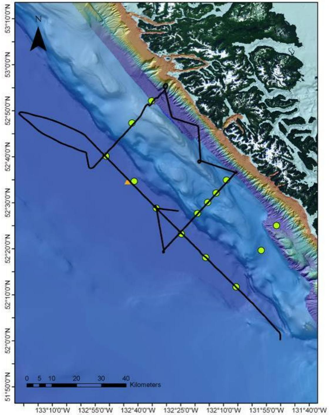
**Figure 3b.** Map of all seismic lines acquired during first refraction experiment. OBS locations from regional grid (green circles) are shown, as well as the ODAS mooring site (orange triangle).
