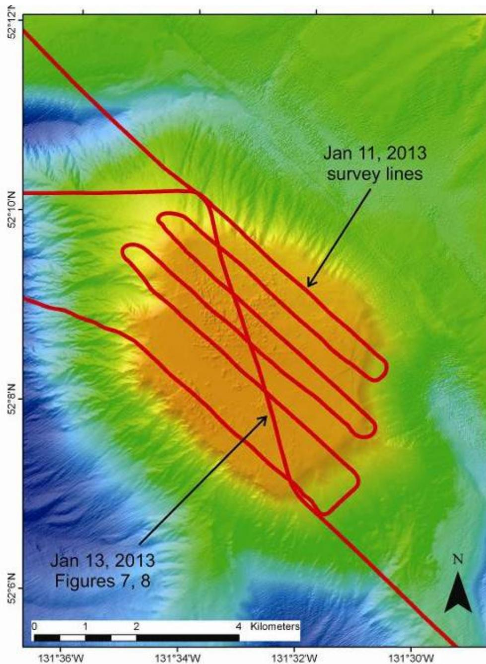
**Figure 3g.** Map of lines acquired across the "plateau"-feature using 3.5 kHz and using the 12 kHz and 18/38 kHz echo sounders.
