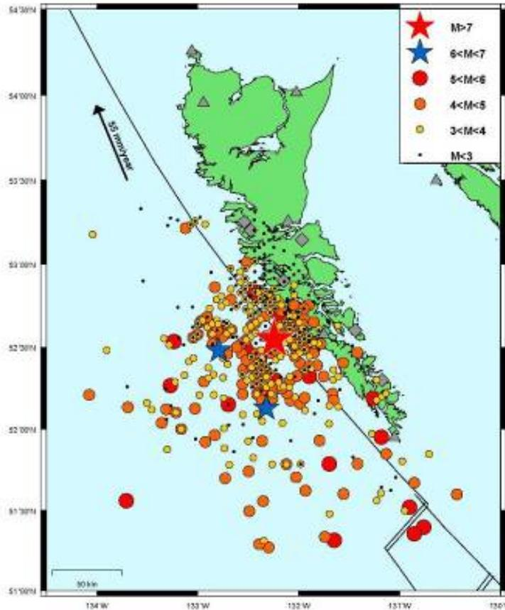
**Figure 1.** Preliminary locations of aftershocks with magnitude 3.0 and above for the first 30 days after the M 7.7 Haida Gwaii earthquake. The epicentre of the main event is shown by the red star and the two largest aftershocks of magnitude 6.0 and above are shown as blue stars (from Cassidy et al., 2012<sup>+</sup>).
