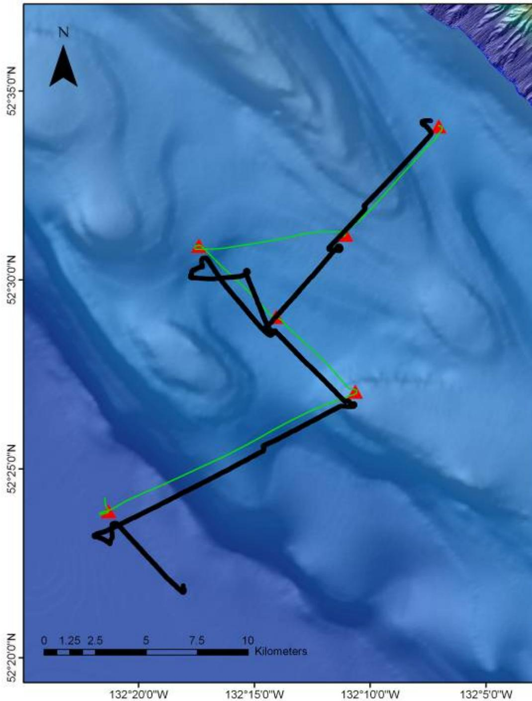
**Figure 3e.** Map of lines during deployment (green) and recovery (black) of the six OBS of second refraction experiment. OBS locations from second refraction experiment are shown as red triangles.
