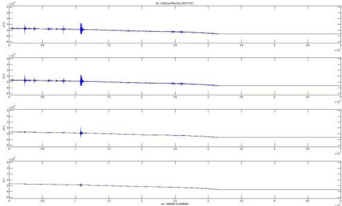
**Figure 9e.** End of recording cycle on OBS #5, Dal-J, from regional grid. Horizontal axis is sample-number (sampling rate is 500 Hz, total record length shown is 1000 seconds). All four channels are shown (ch1: hydrophone; ch2: vertical; ch3=horizontal 1; ch4: horizontal 2).
