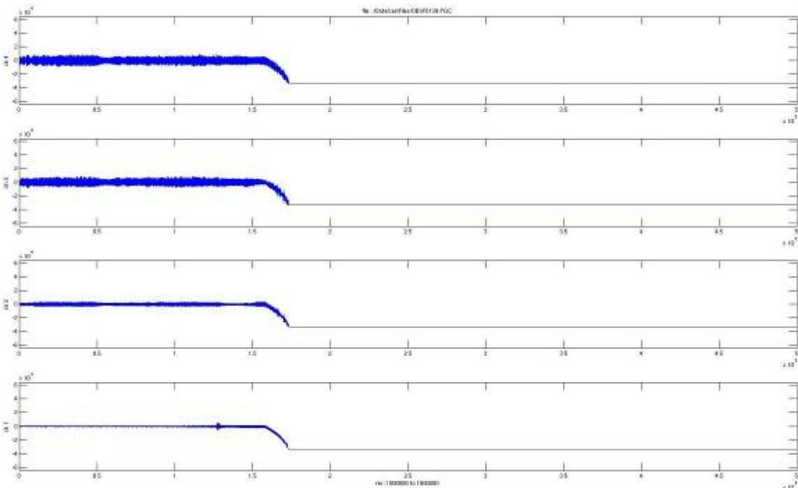
**Figure 9f.** End of recording cycle on OBS #6, NRCan-F, from regional grid. Horizontal axis is sample-number (sampling rate is 500 Hz, total record length shown is 1000 seconds). All four channels are shown (ch1: hydrophone; ch2: vertical; ch3=horizontal 1; ch4: horizontal 2).
