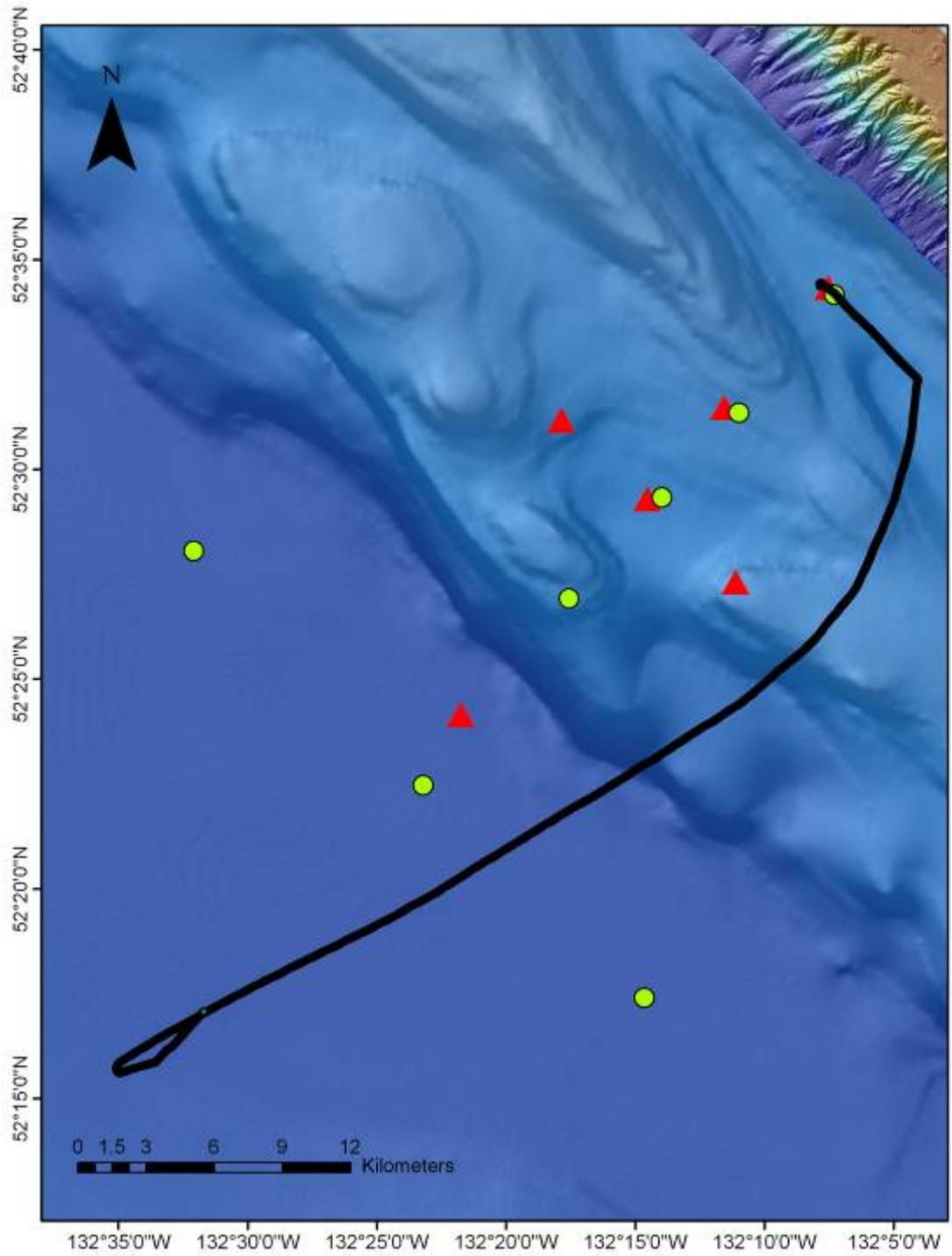
**Figure 3f.** Map of line where only 3.5 kHz data were acquired during operational downtimes between 2nd refraction experiment OBS deployment and start of airgun work. OBS locations from regional grid are shown in green circles, OBS locations from second refraction experiment are shown as red triangles.
