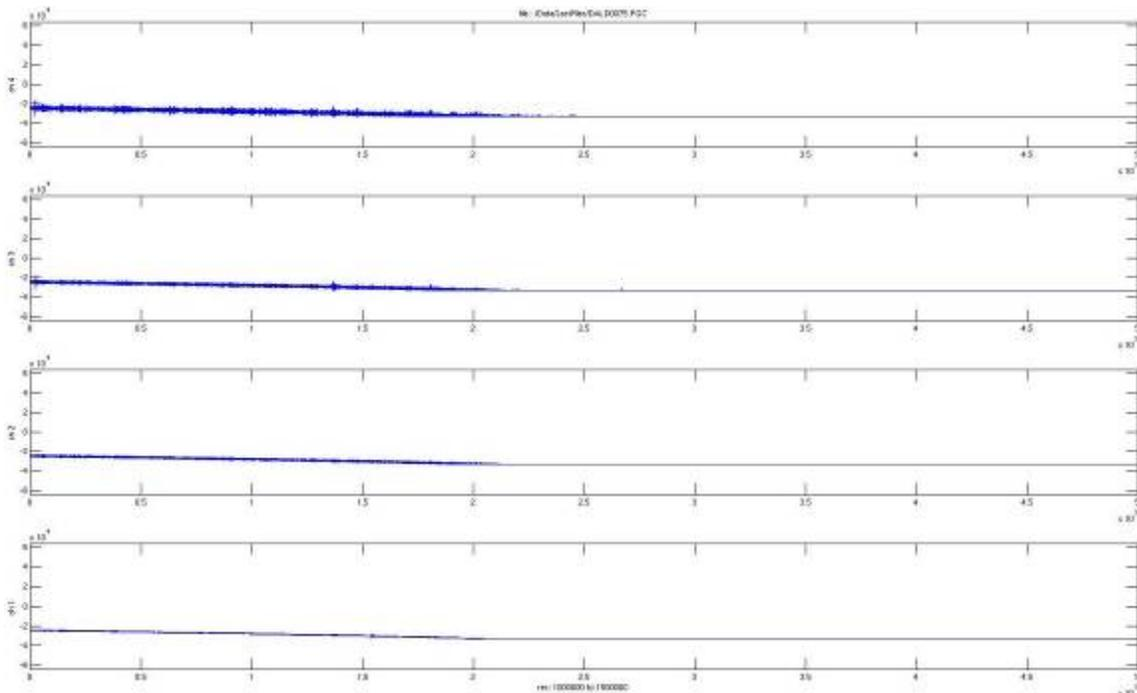
**Figure 9g.** End of recording cycle on OBS #7, Dal-D, from regional grid. Horizontal axis is sample-number (sampling rate is 500 Hz, total record length shown is 1000 seconds). All four channels are shown (ch1: hydrophone; ch2: vertical; ch3=horizontal 1; ch4: horizontal 2).
