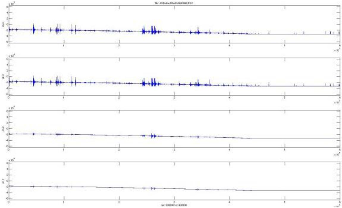
**Figure 9i.** End of recording cycle on OBS #9, Dal-B, from regional grid. Horizontal axis is sample-number (sampling rate is 500 Hz, total record length shown is 1000 seconds). All four channels are shown (ch1: hydrophone; ch2: vertical; ch3=horizontal 1; ch4: horizontal 2).
