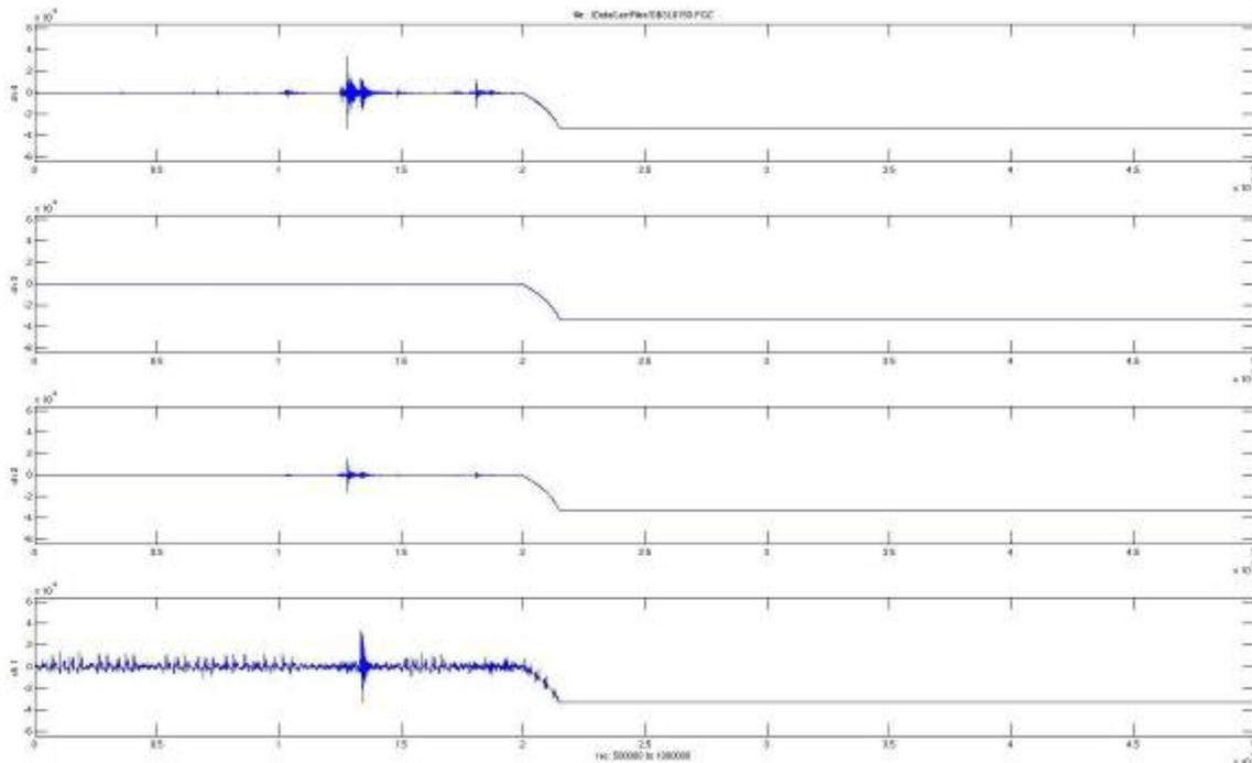
**Figure 9h.** End of recording cycle on OBS #8, NRCan-L, from regional grid. Horizontal axis is sample-number (sampling rate is 500 Hz, total record length shown is 1000 seconds). All four channels are shown (ch1: hydrophone; ch2: vertical; ch3=horizontal 1; ch4: horizontal 2).
