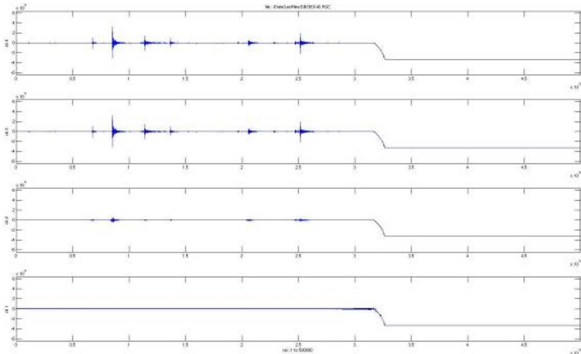
**Figure 9k.** End of recording cycle on OBS #11, NRCan-E, from regional grid. Horizontal axis is sample-number (sampling rate is 500 Hz, total record length shown is 1000 seconds). All four channels are shown (ch1: hydrophone; ch2: vertical; ch3=horizontal 1; ch4: horizontal 2).
