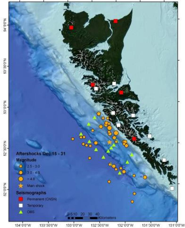
**Figure 2.** Map of OBS stations deployed during cruise 2012005PGC and location of land seismometers. Locations with magnitude of aftershocks recorded only using the land stations during the actual active recording period of the 14 OBS are shown in orange dots (for magnitude scale, see legend).
