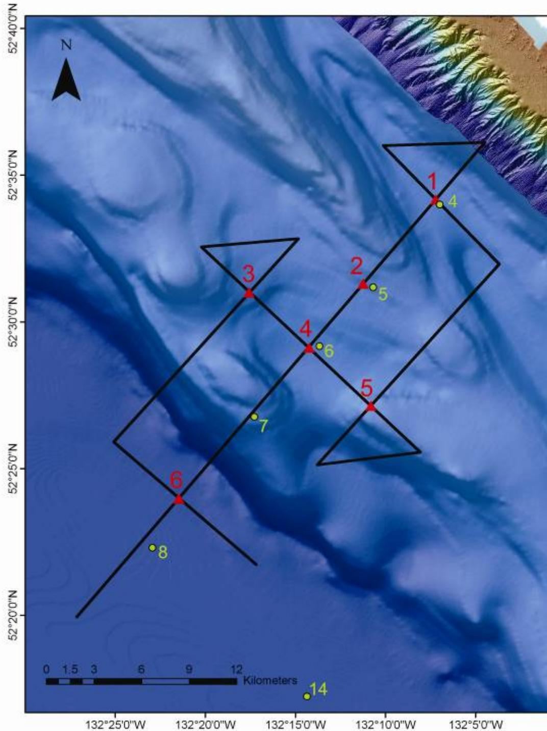
**Figure 3d.** Map of seismic lines acquired during second refraction experiment. OBS locations from regional grid (green circles) and 2nd refraction experiment (red triangles) are shown and label represents station numbers as listed in Tables 1 and 4.
