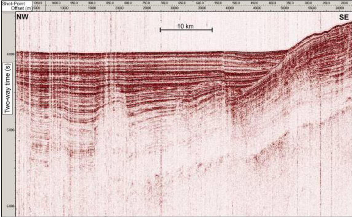
**Figure 5.** Example of airgun data recorded on single-channel streamer.
