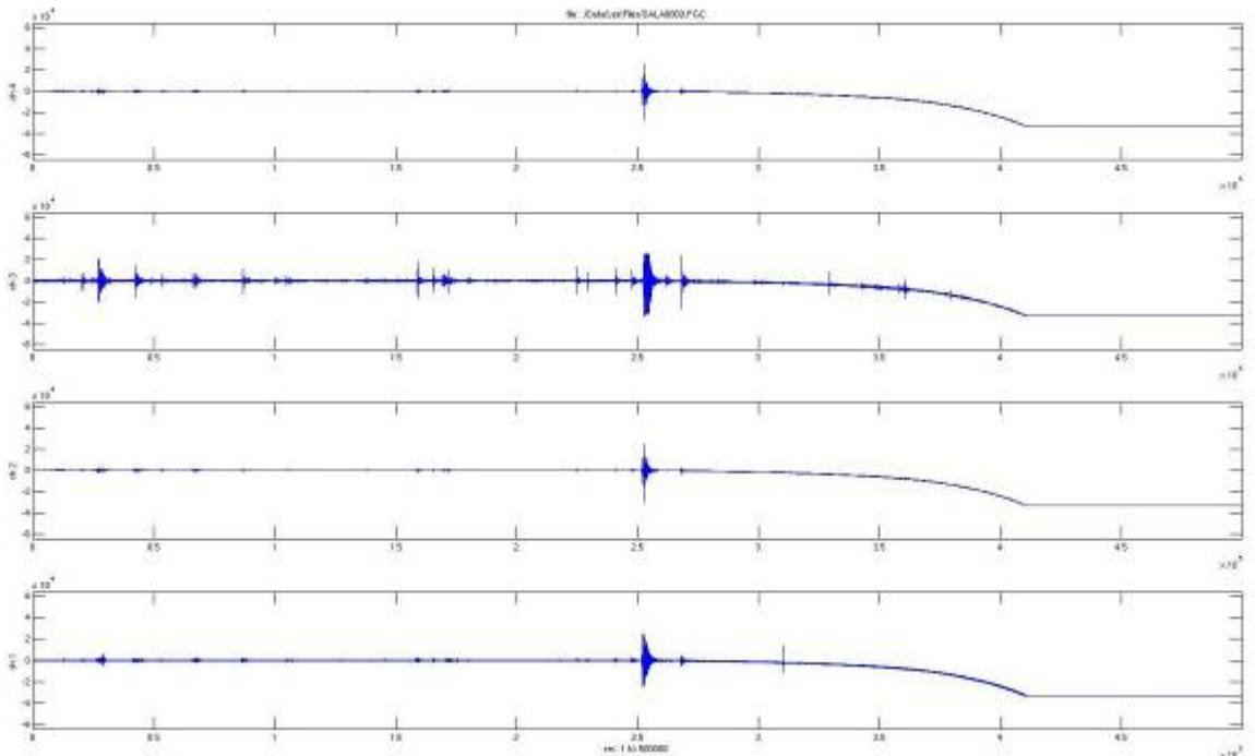
**Figure 9j.** End of recording cycle on OBS #10, Dal-A, from regional grid. Horizontal axis is sample-number (sampling rate is 500 Hz, total record length shown is 1000 seconds). All four channels are shown (ch1: hydrophone; ch2: vertical; ch3=horizontal 1; ch4: horizontal 2).
