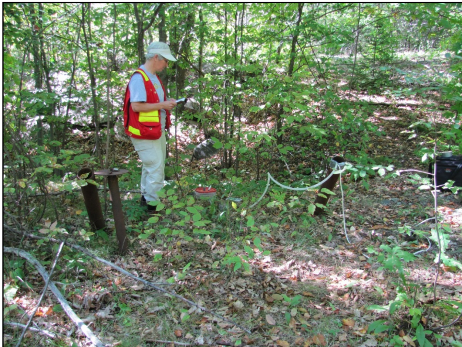
Figure 5: (a) Groundwater sampling from the adit at the Amalgamated Rare Earth No. 2 Mine; (b) Sampling from a diamond drill hole at the Croft South Zone.
