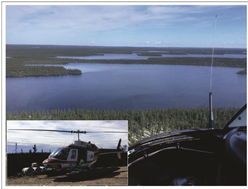
Figure 3 A Bell 206B (Jet Ranger) helicopter on floats (inset) on approach to a typical lake (1 to 5 km 2 ) for sampling. Pre-labelled synthetic cloth bags and high-density polyethylene (HDPE) bottles are used to collect (approximately) a 1-kg sample of lake sediment and a 250-ml sample of surface lake water.
