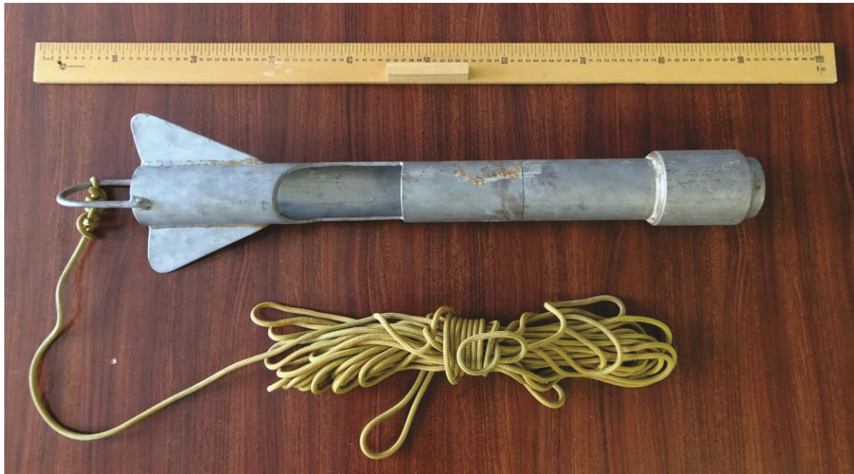
Figure 2 About 1 kg of wet lake sediment (gyttja) is collected by dropping the sampler (above) from a platform attached to the landing skid opposite the pilot. Ideally, the entire length of the weighted sampler penetrates the lake bottom sediments to a depth below the sediment-water interface so that the upper layers of gyttja are forced out the vent located towards the tail of the sampler, reducing the possibility of contamination of the sample by recent (Anthropocene) sources.
