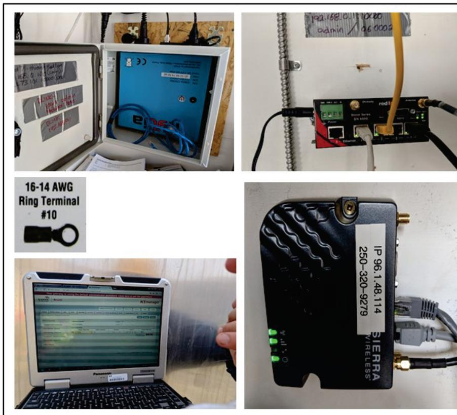
**Fig. 6** Geocoordinators, routers and modems in bungalows: ring terminals used for attachment to power sources (centre left); Ripley Landslide COORD-00007 (top left, NRCan photo 2020-316); Red Lion Router at Ripley Landslide (top right, NRCan photo 2020-317); D Link Router at South Slide (bottom right, NRCan photo 2020-318); ACE management software on laptop (bottom left, NRCan photo 2020-319).
