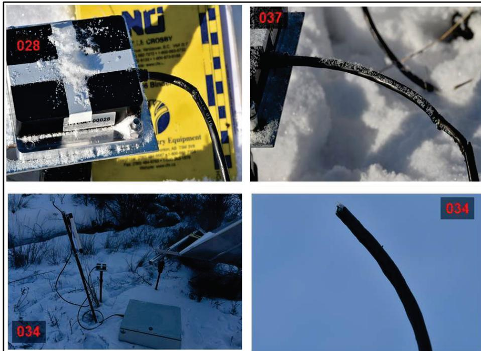
**Fig. 7** Cables to Geocubes and battery boxes are at risk from damage by wildlife: damage to Geocube KYL 028 (top left, NRCan photo 2020-320); damage to Geocube KYL 037 (top right, NRCan photo 2020-321); damage to Geocube KYL 034 (bottom left, NRCan photo 2020-322); detail of damage to Geocube KYL 034 cable (bottom right, NRCan photo 2020-323). Cameras were installed in 2017 to monitor instruments on the landslide and determine which animals were damaging wires and other components.
