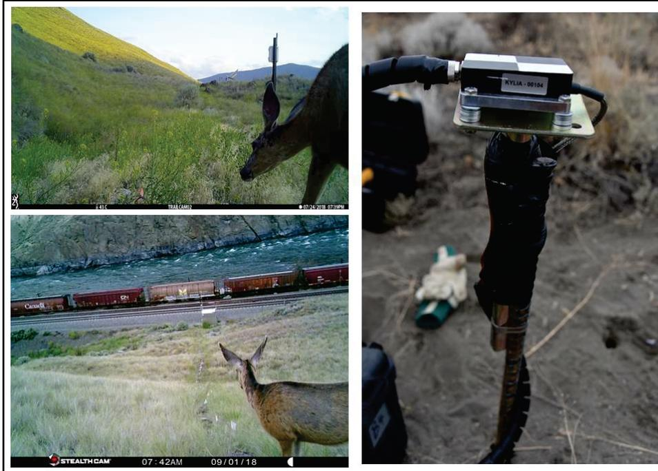
**Fig. 8** Deer appear to be the dominant animal crossing the landslide and damaging cables, either by chewing or rutting with antlers. Wiring is now protected with a combination of steel meshing, plastic wrapping and rubberized adhesive electrical tape (NRCan photo 2020-324). Time will tell whether this approach is effective.
