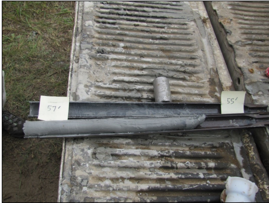
Figure A-23: Split-spoon core sample from the stratigraphic borehole interval 55-57 ft. Photograph by A.J. Desbarats. NRCan Photo Database number 2020-663.
