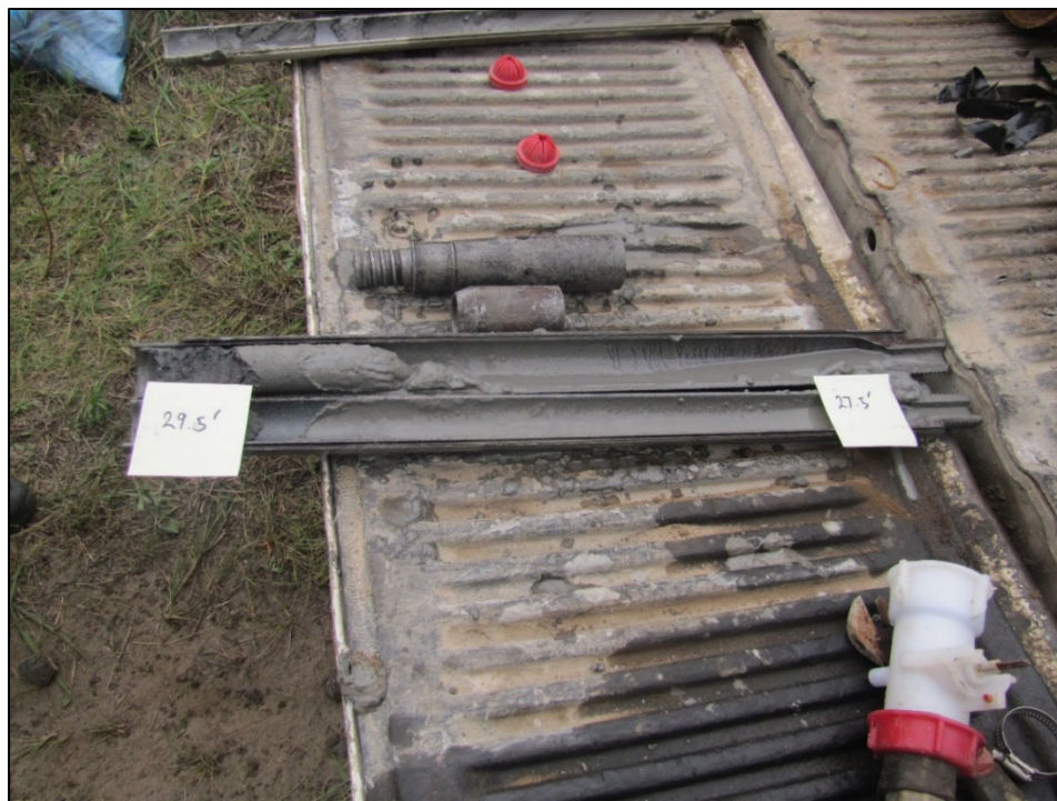
Figure A-12: Split-spoon core sample from the stratigraphic borehole interval 27.5-29.5 ft. Photograph by A.J. Desbarats. NRCan Photo Database number 2020-652.
