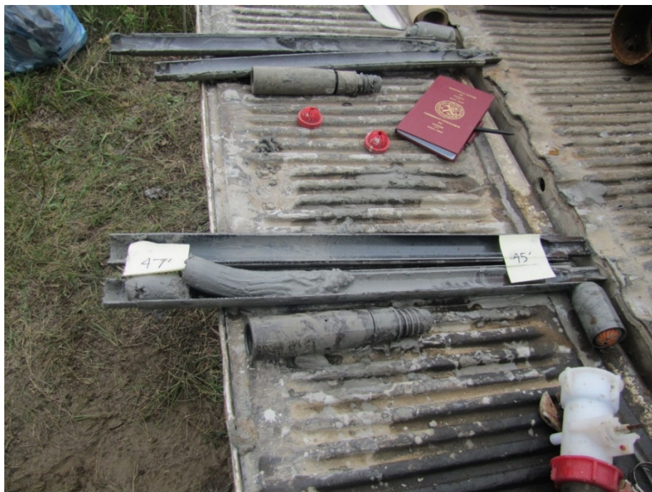
Figure A-19: Split-spoon core sample from the stratigraphic borehole interval 45-47 ft. Photograph by A.J. Desbarats. NRCan Photo Database number 2020-659.
