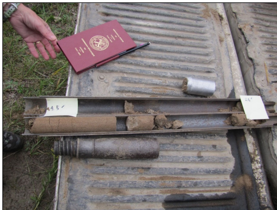
Figure A-2: Split-spoon core sample from the stratigraphic borehole interval 2.5-4.5 ft. Photograph by A.J. Desbarats. NRCan Photo Database number 2020-643.
