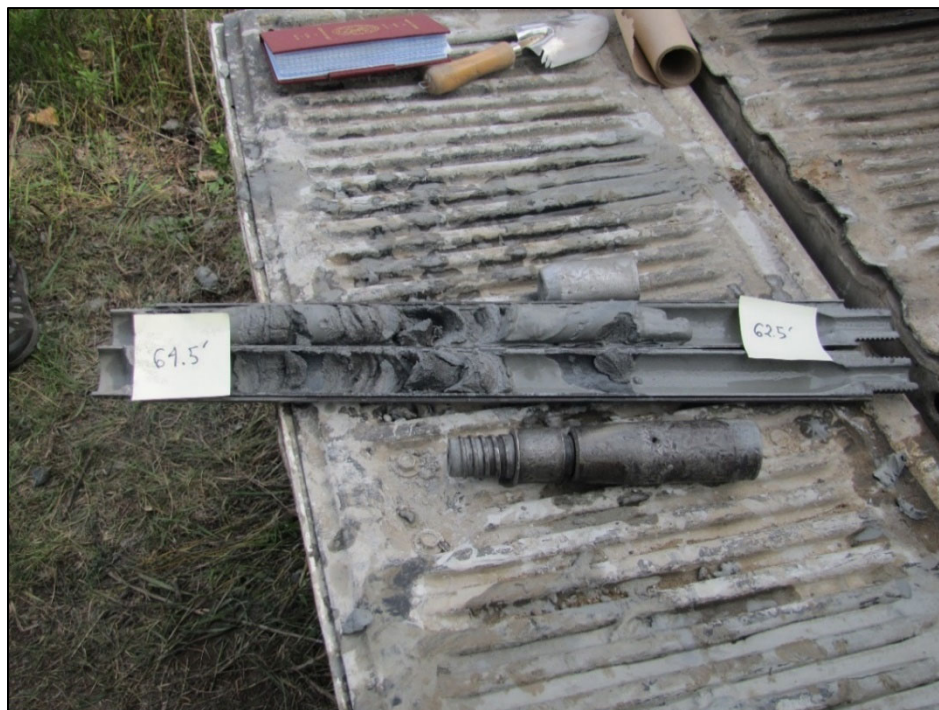
Figure A-26: Split- spoon core sample from the stratigraphic borehole interval 62.5-64.5 ft. Photograph by A.J. Desbarats. NRCan Photo Database number 2020-666.
