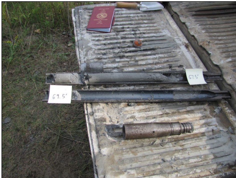
Figure A-28: Split-spoon core sample from the stratigraphic borehole interval 67.5-69.5 ft. Photograph by A.J. Desbarats. NRCan Photo Database number 2020-668.
