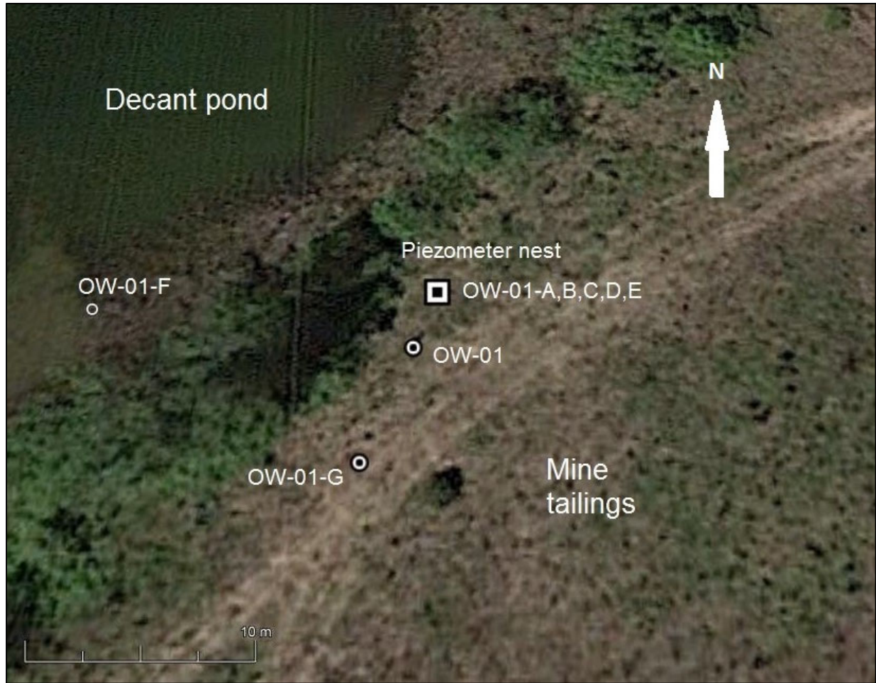
Figure 5: Layout of piezometers and observation wells in the tailings impoundment southeast of the decant pond. OW-01 coordinates: longitude -74.02625° W and latitude 45.504555° N. Google Earth image used with permission.
