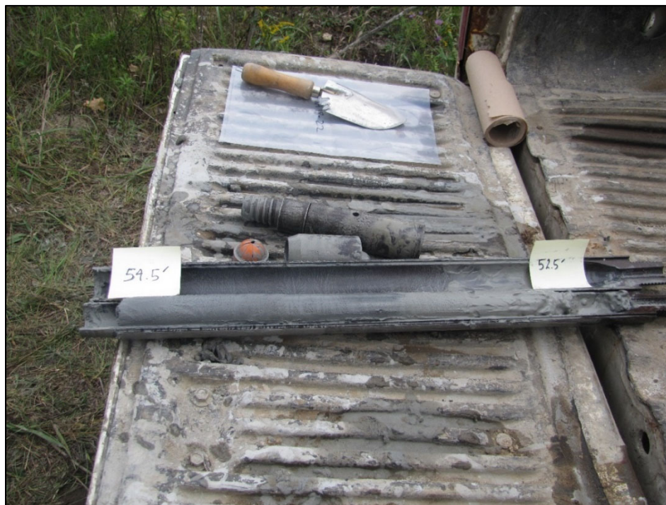
Figure A-22: Split-spoon core sample from the stratigraphic borehole interval 52.5-54.5 ft. Photograph by A.J. Desbarats. NRCan Photo Database number 2020-662.
