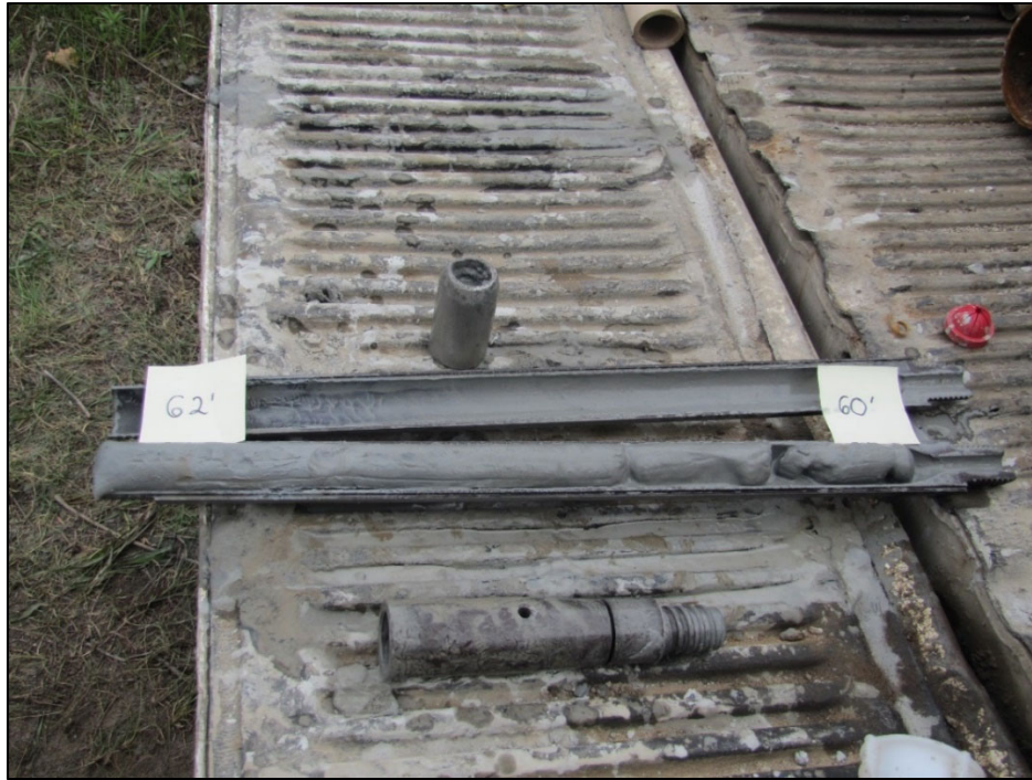
Figure A-25: Split- spoon core sample from the stratigraphic borehole interval 60-62 ft. Photograph by A.J. Desbarats. NRCan Photo Database number 2020-665.
