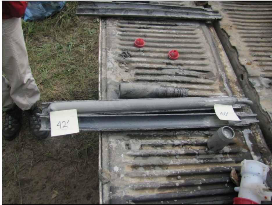
Figure A-17: Split-spoon core sample from the stratigraphic borehole interval 40-42 ft. Photograph by A.J. Desbarats. NRCan Photo Database number 2020-657.
