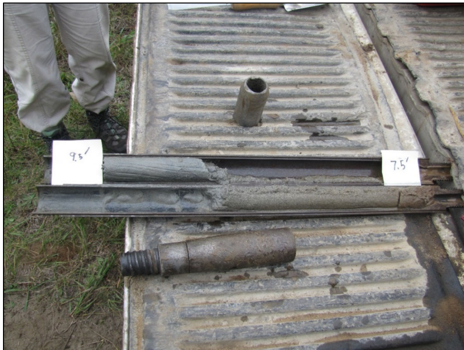
Figure A-4: Split-spoon core sample from the stratigraphic borehole interval 7.5-9.5 ft. Photograph by A.J. Desbarats. NRCan Photo Database number 2020-645.
