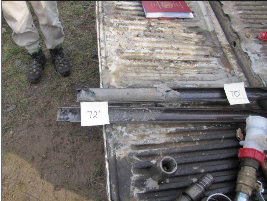
Figure A-29: Split-spoon core sample from the stratigraphic borehole interval 70-72 ft. Photograph by A.J. Desbarats. NRCan Photo Database number 2020-669.
