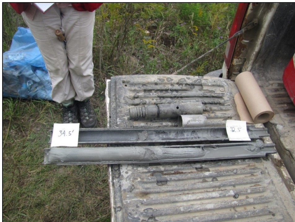
Figure A-14: Split-spoon core sample from the stratigraphic borehole interval 32.5-34.5 ft. Photograph by A.J. Desbarats. NRCan Photo Database number 2020-654.
