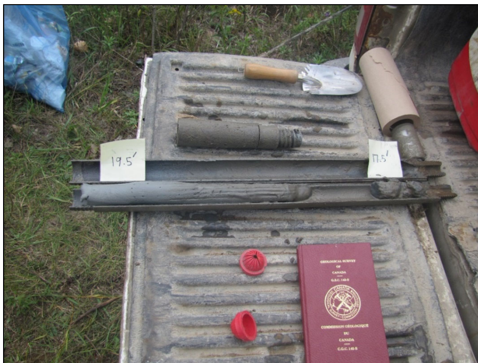
Figure A-8: Split- spoon core sample from the stratigraphic borehole interval 17.5-19.5 ft. Photograph by A.J. Desbarats. NRCan Photo Database number 2020-648.
