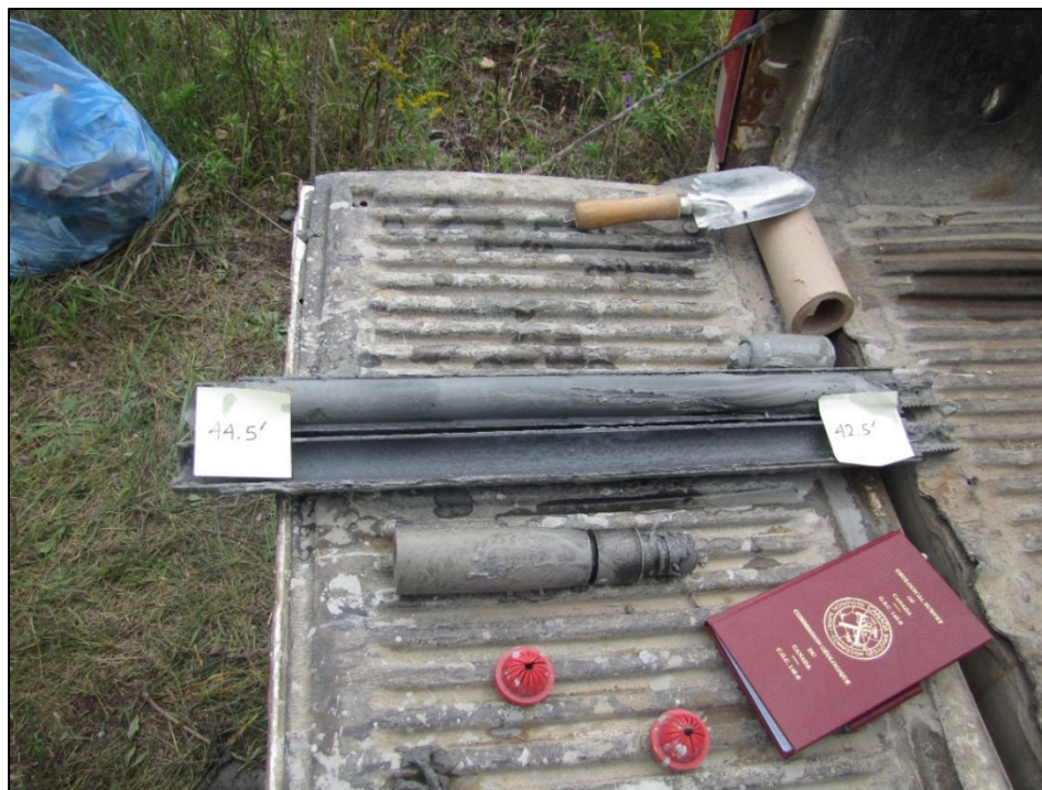
Figure A-18: Split-spoon core sample from the stratigraphic borehole interval 42.5-44.5 ft. Photograph by A.J. Desbarats. NRCan Photo Database number 2020-658.
