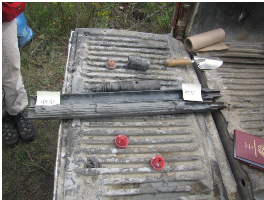
Figure A-20: Split-spoon core sample from the stratigraphic borehole interval 47.5-49.5 ft. Photograph by A.J. Desbarats. NRCan Photo Database number 2020-660.
