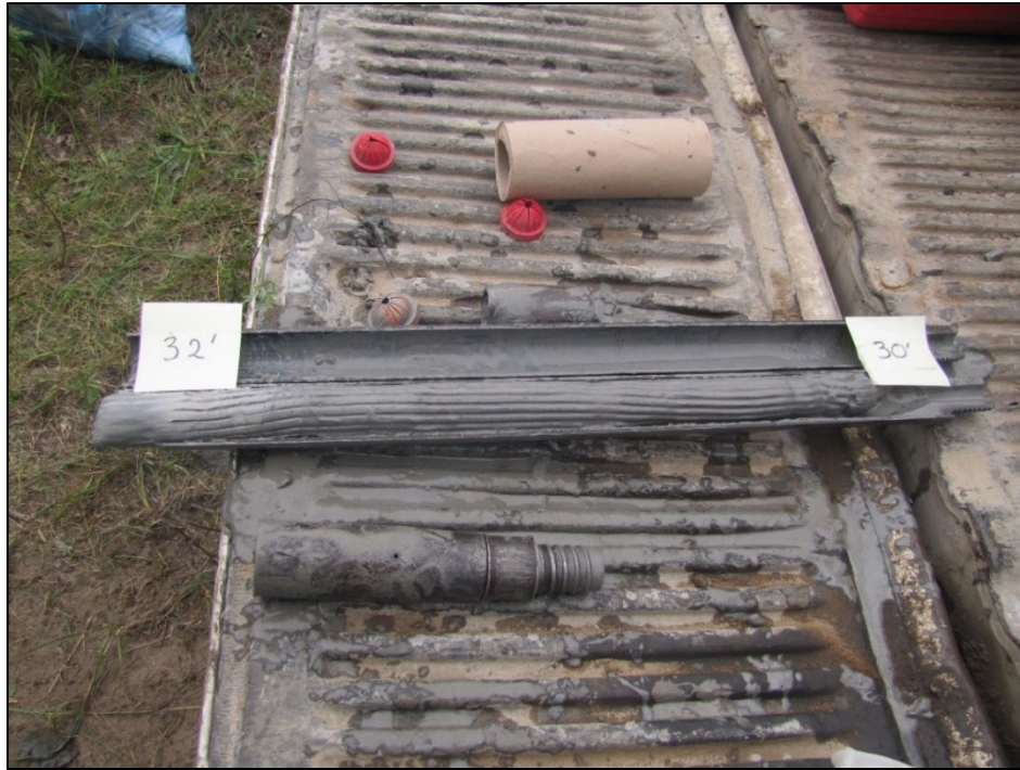
Figure A-13: Split-spoon core sample from the stratigraphic borehole interval 30-32 ft. Photograph by A.J. Desbarats. NRCan Photo Database number 2020-653.
