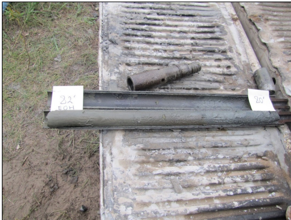
Figure A-32: Split-spoon core sample from the stratigraphic borehole interval 80-82 ft. Photograph by A.J. Desbarats. NRCan Photo Database number 2020-672.
