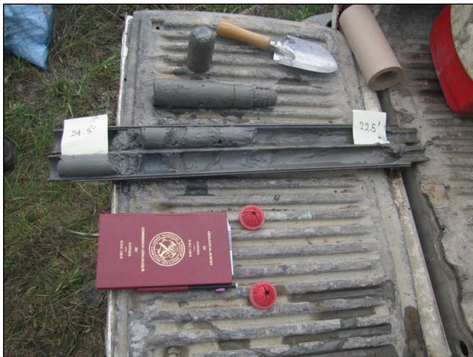
Figure A-10: Split-spoon core sample from the stratigraphic borehole interval 22.5-24.5 ft. Photograph by A.J. Desbarats. NRCan Photo Database number 2020-650.
