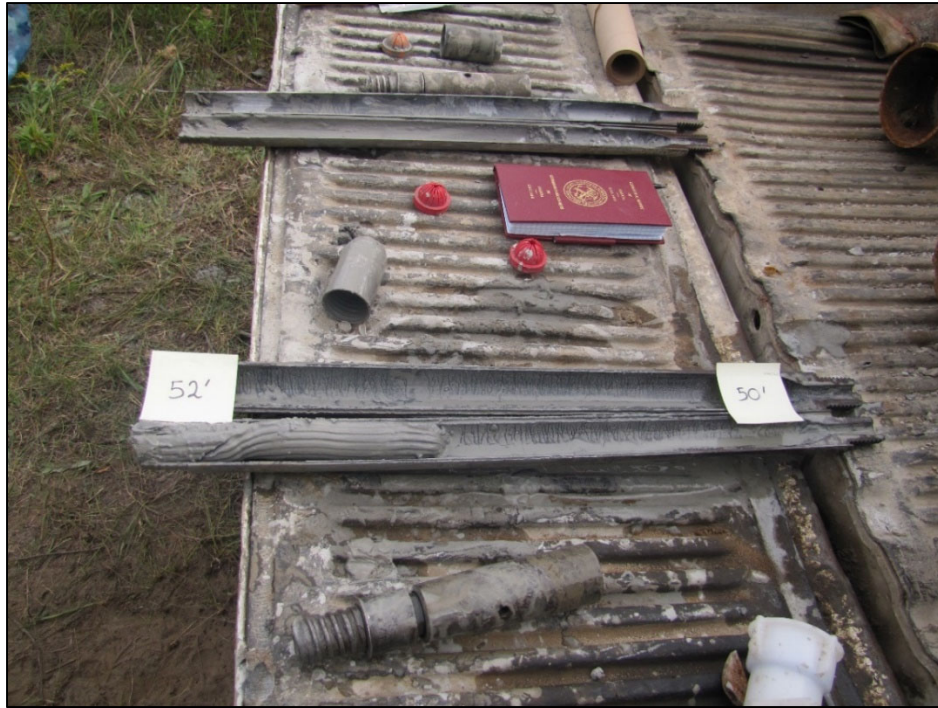
Figure A-21: Split-spoon core sample from the stratigraphic borehole interval 50-52 ft. Photograph by A.J. Desbarats. NRCan Photo Database number 2020-661.
