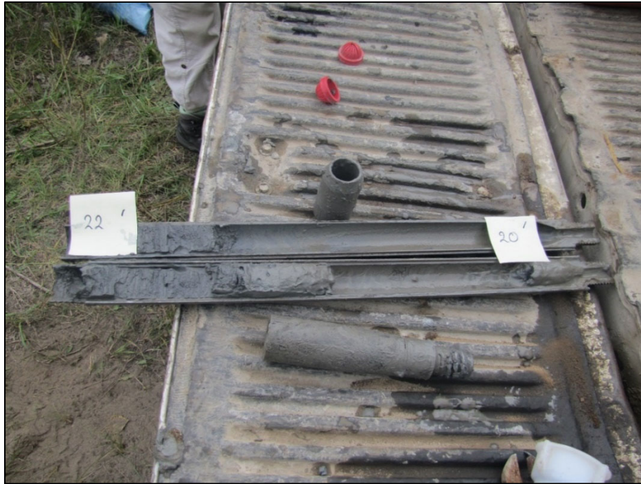
Figure A-9: Split-spoon core sample from the stratigraphic borehole interval 20-22 ft. Photograph by A.J. Desbarats. NRCan Photo Database number 2020-649.
