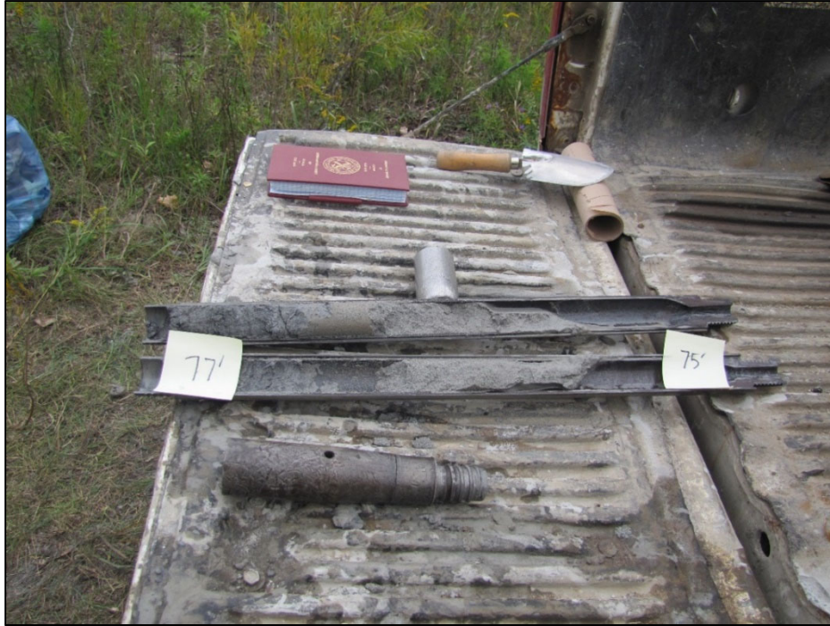
Figure A-31: Split-spoon core sample from the stratigraphic borehole interval 75-77 ft. Photograph by A.J. Desbarats. NRCan Photo Database number 2020-671.
