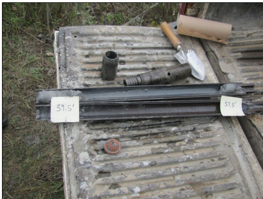
Figure A-24: Split-spoon core sample from the stratigraphic borehole interval 57.5-59.5 ft. Photograph by A.J. Desbarats. NRCan Photo Database number 2020-664.
