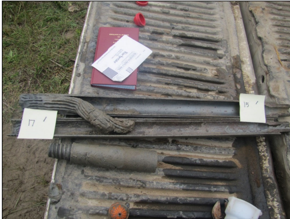
Figure A-7: Split- spoon core sample from the stratigraphic borehole interval 15-17 ft. Photograph by A.J. Desbarats. NRCan Photo Database number 2020-647.
