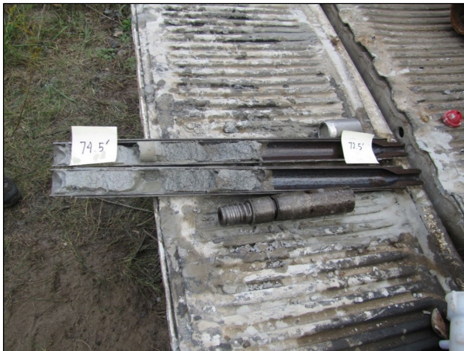
Figure A-30: Split-spoon core sample from the stratigraphic borehole interval 72.5-74.5 ft. Photograph by A.J. Desbarats. NRCan Photo Database number 2020-670.
