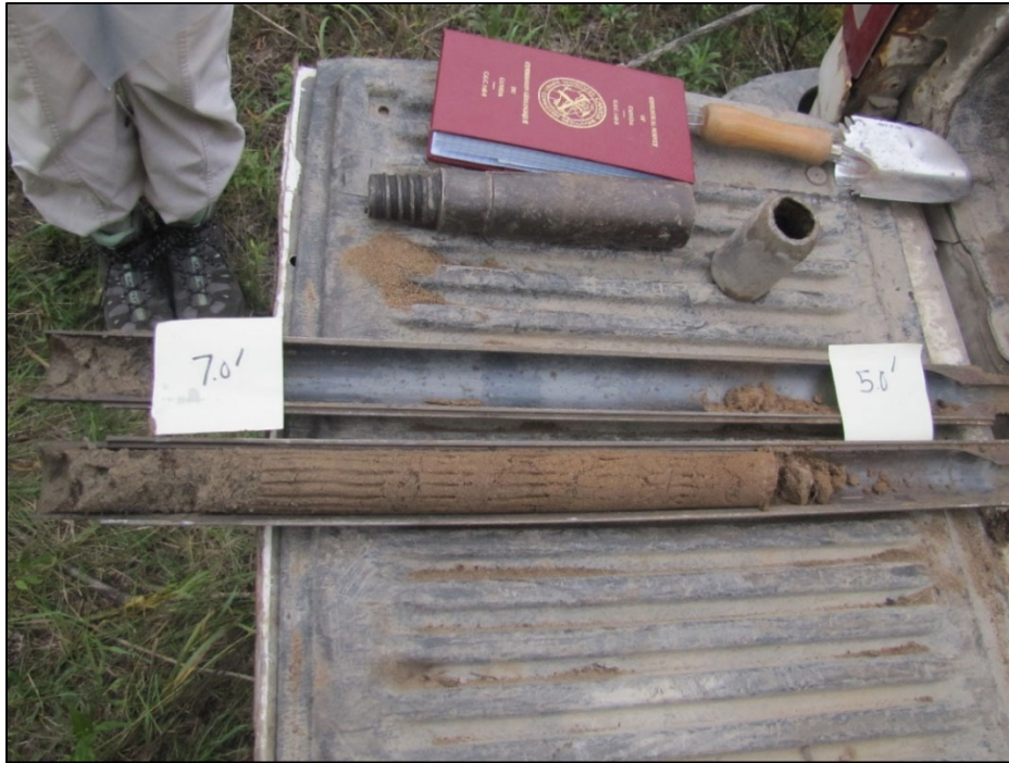
Figure A-3: Split-spoon core sample from the stratigraphic borehole interval 5-7 ft. Photograph by A.J. Desbarats. NRCan Photo Database number 2020-644.
