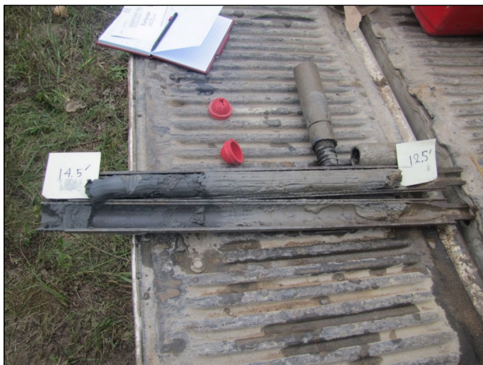
Figure A-6: Split-spoon core sample from the stratigraphic borehole interval 12.5-14.5 ft. Photograph by A.J. Desbarats. NRCan Photo Database number 2020-646.
