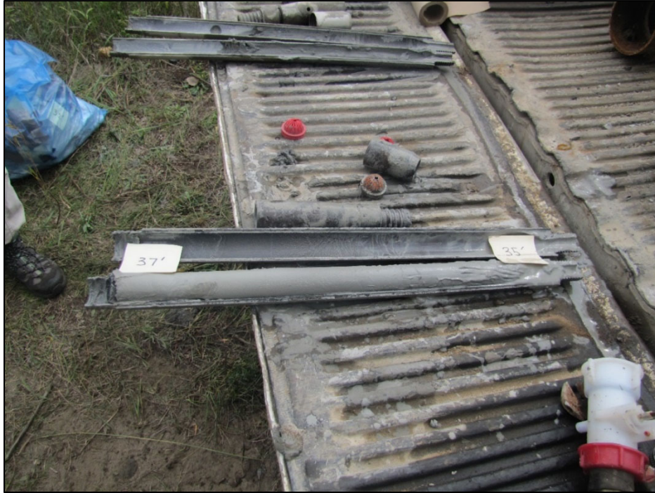
Figure A-15: Split-spoon core sample from the stratigraphic borehole interval 35-37 ft. Photograph by A.J. Desbarats. NRCan Photo Database number 2020-655.
