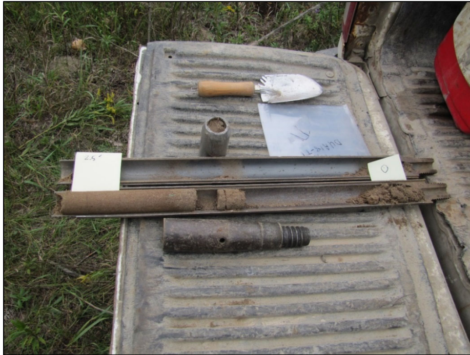
Figure A-1: Split-spoon core sample from the stratigraphic borehole interval 0-2.5 ft. Photograph by A.J. Desbarats. NRCan Photo Database number 2020-642.
