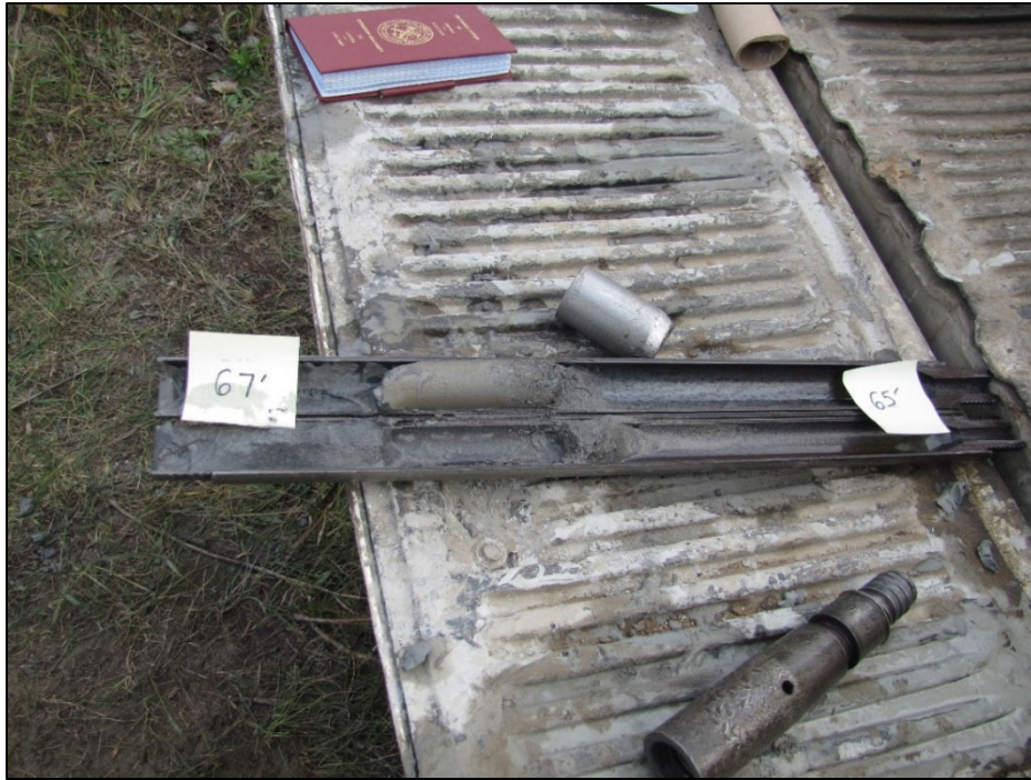
Figure A-27: Split-spoon core sample from the stratigraphic borehole interval 65-67 ft. Photograph by A.J. Desbarats. NRCan Photo Database number 2020-667.
