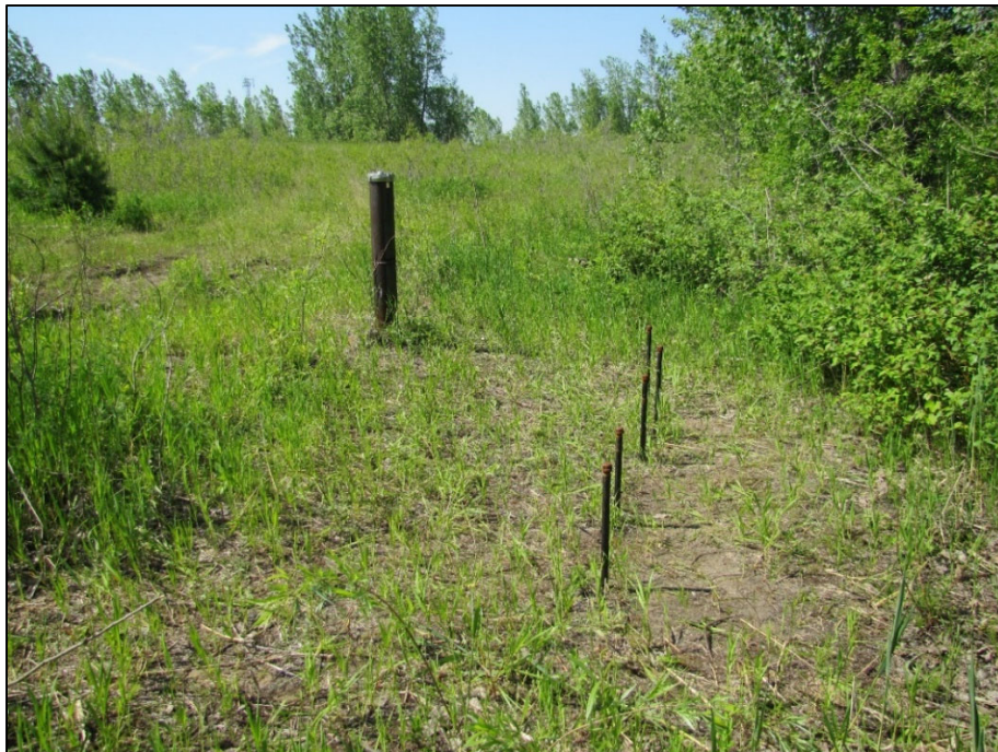
Figure 7: Piezometers OW-01-A, B, C, D, E. Observation well OW-01 is in the background. Photograph by A.J. Desbarats. NRCan Photo Database number 2020-636.
