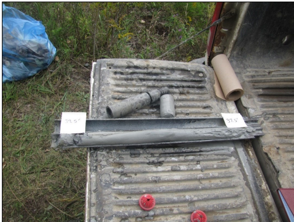
Figure A-16: Split-spoon core sample from the stratigraphic borehole interval 37.5-39.5 ft. Photograph by A.J. Desbarats. NRCan Photo Database number 2020-656.
