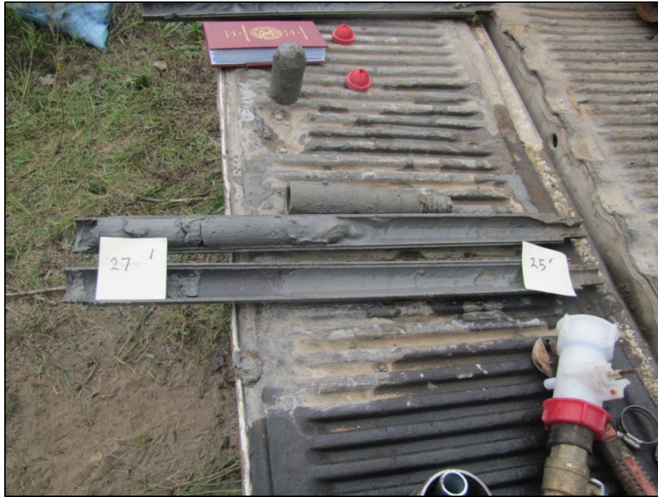
Figure A-11: Split-spoon core sample from the stratigraphic borehole interval 25-27 ft. Photograph by A.J. Desbarats. NRCan Photo Database number 2020-651.
