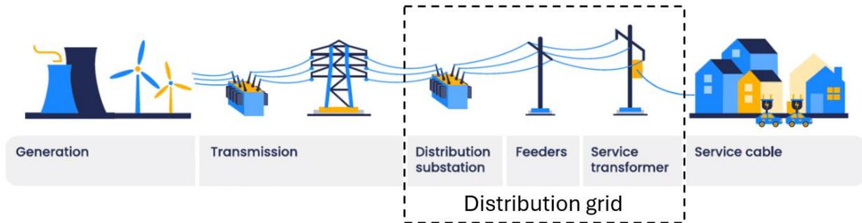
As fleets begin to electrify, they will cause a certain level of power demand as they charge. If that demand exceeds the capacity that is available on the distribution grid, upgrades to the system are needed. There are two main distribution grid upgrades that vary in cost based on the capacity required and the type of upgrade needed:
