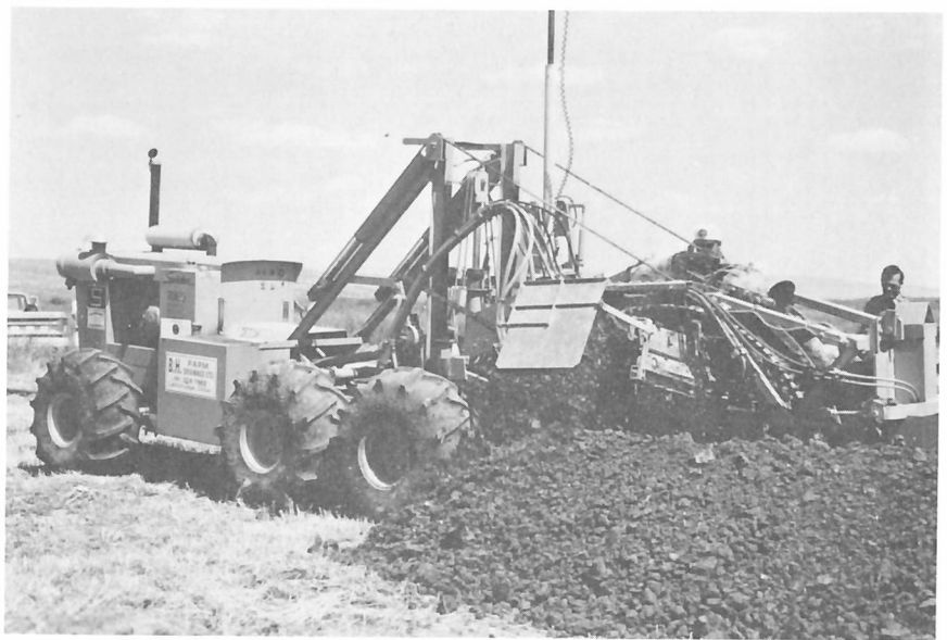
FIG. 14 Wheel trencher for installing subsurface drains.
