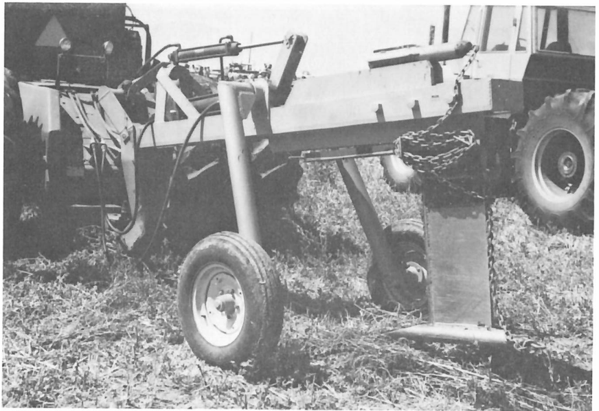
FIG. 13 Plow used for forming mole drains.
