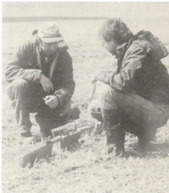
The EM38 conductivity meter is used to assess salinity in the field.
