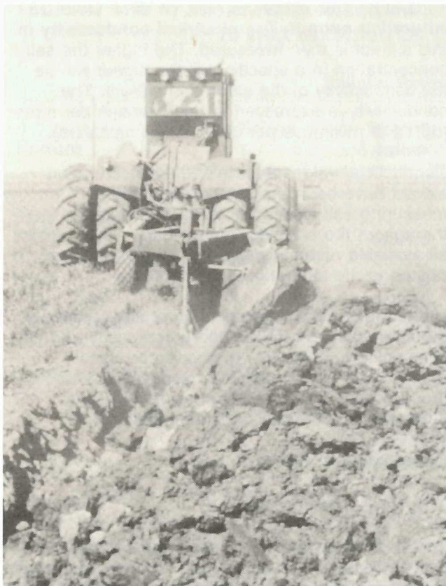
Deep plowing is expensive but breaks up the hardpan and brings up calcium to help reclaim true solonchic soils. Deep plowing is not recommended for saline soils.
