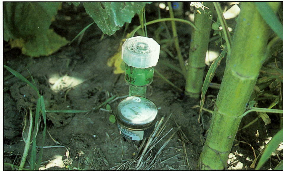
Tension meters used to measure soil moisture tension to aid in the proper scheduling of irrigation.
