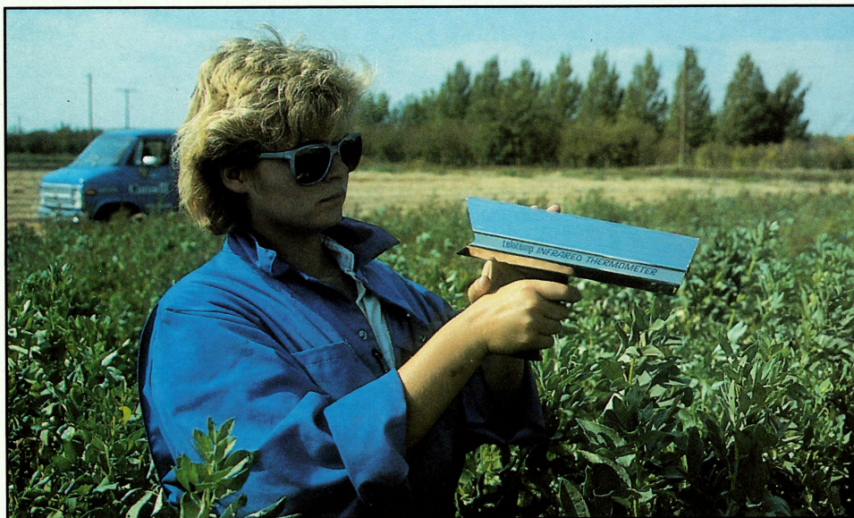
Infrared thermometer to measure the temperature of the crops canopy. By relating this figure to the temperature of the air, it can be determined if the crop is under stress.
