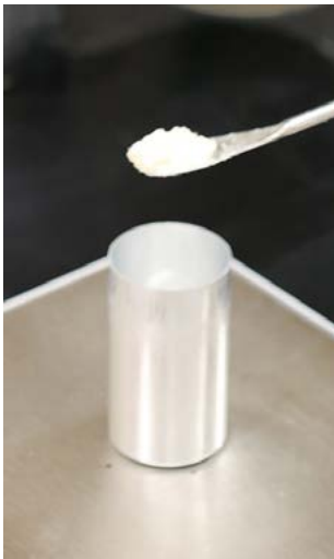
Weigh 4 g (14% mc) into RVA canister
