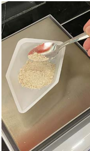
Weigh two 7 g (14% mc) ground samples into long tubes
