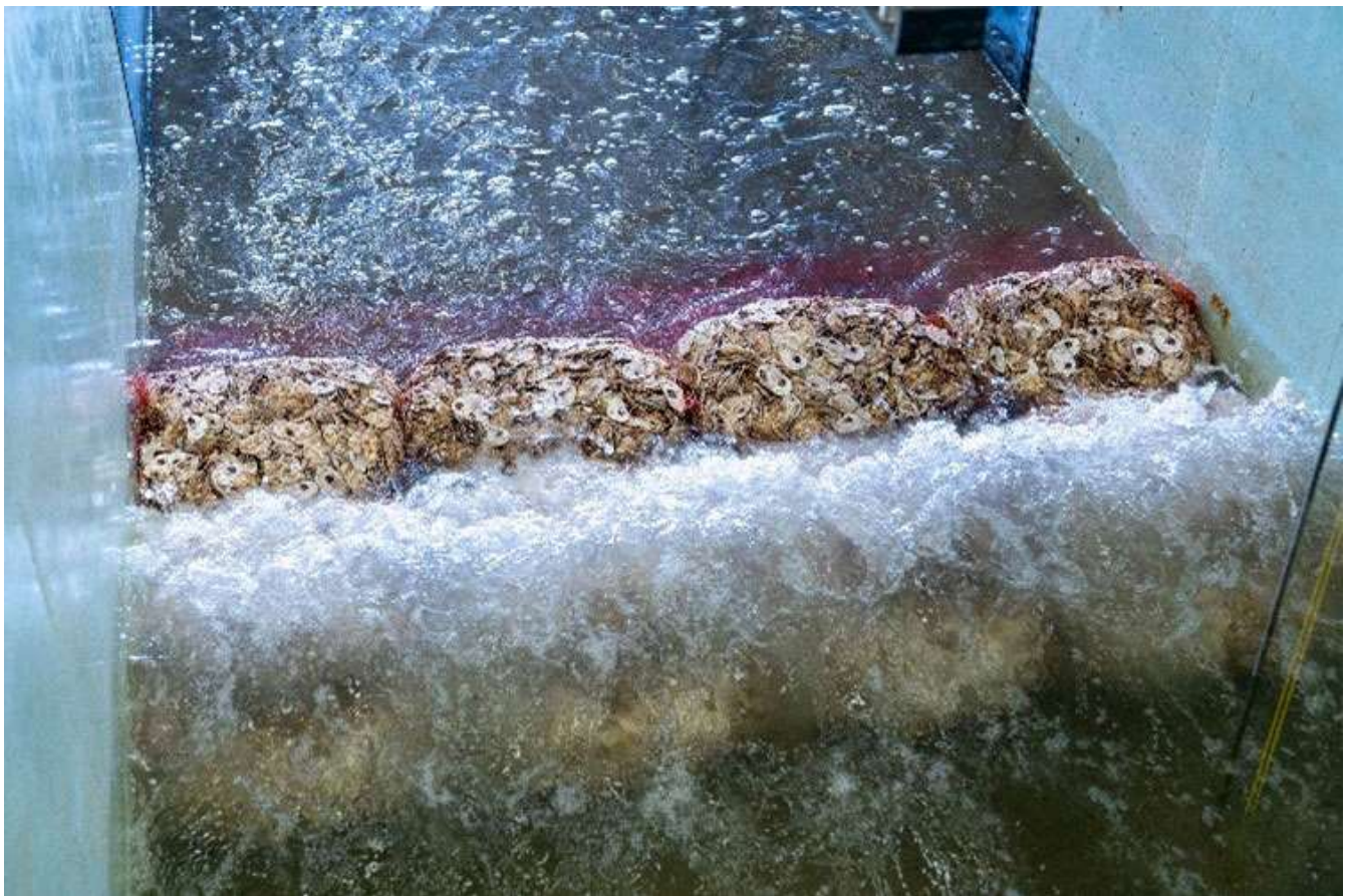
A nature-based emergency flood barrier made of oyster-shell filled biodegradable bags.
