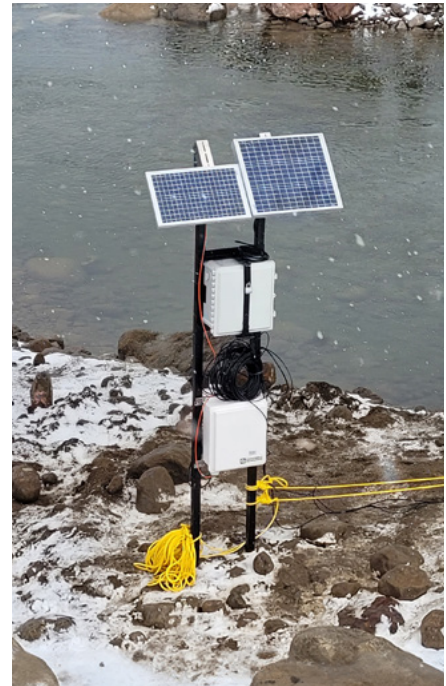
Data acquisition system used to register water quality and flow data from the Duval River in Pangnirtung.
