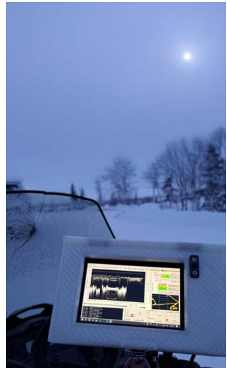
Ice-penetrating radar processing software operates on a snowmobile-mounted console. Photo credit: Winter Trails project team
