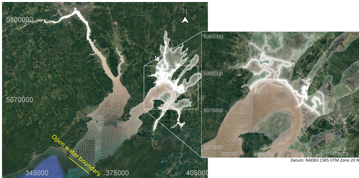
Figure 4.1 Model mesh and boundary with a detailed inset of upper Cumberland Basin
