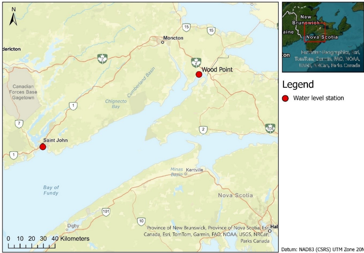
Figure 2.10. Location of water level stations in the Bay of Fundy, where tidal gauge #65 at Saint John is managed by the CHS and water level gauge at Wood Point is managed by SMU.
